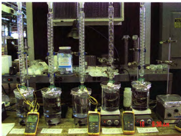
Figure 26. Bench top test setup for Al coupon corrosion tests at 140 F and with 2500 ppm B and the pH=9.4 or 8.0.
