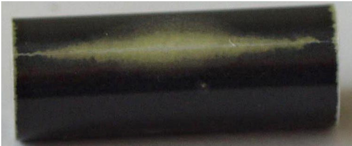
Figure 82. Outer surface of scratched ZIRLO sample following oxidation at 985^{\circ}\text{C} for 3400 s. The local hydrogen pickup under the yellow surface is 440 wppm.
