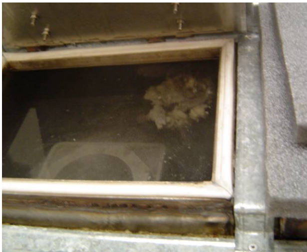
Figure 7: Flotation of Part of Debris Bed
