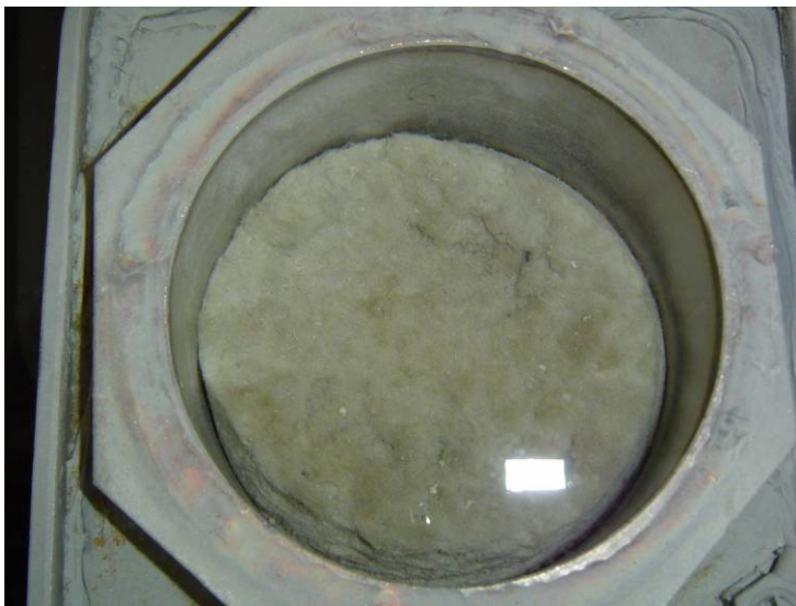
Figure 13: Debris Bed With Warping Around Circumference
