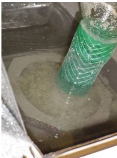
Figure 9: Debris Bed Filling to Top of Chimney
