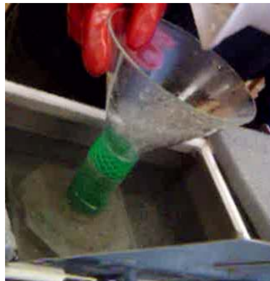
Figure 10: Re-Poured Debris Bed Mounding Above Top of Chimney
