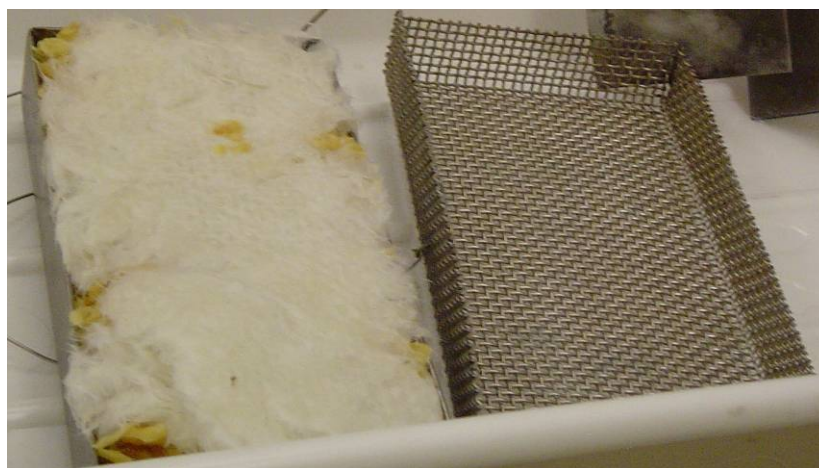
Figure 11: Sample Basket with Densely Packed Layers of Debris
