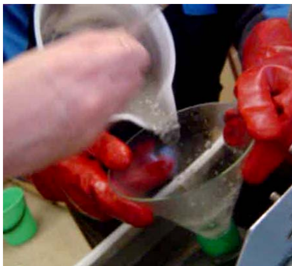
Figure 4: Agglomerated Debris Being Poured Onto Test Screen
