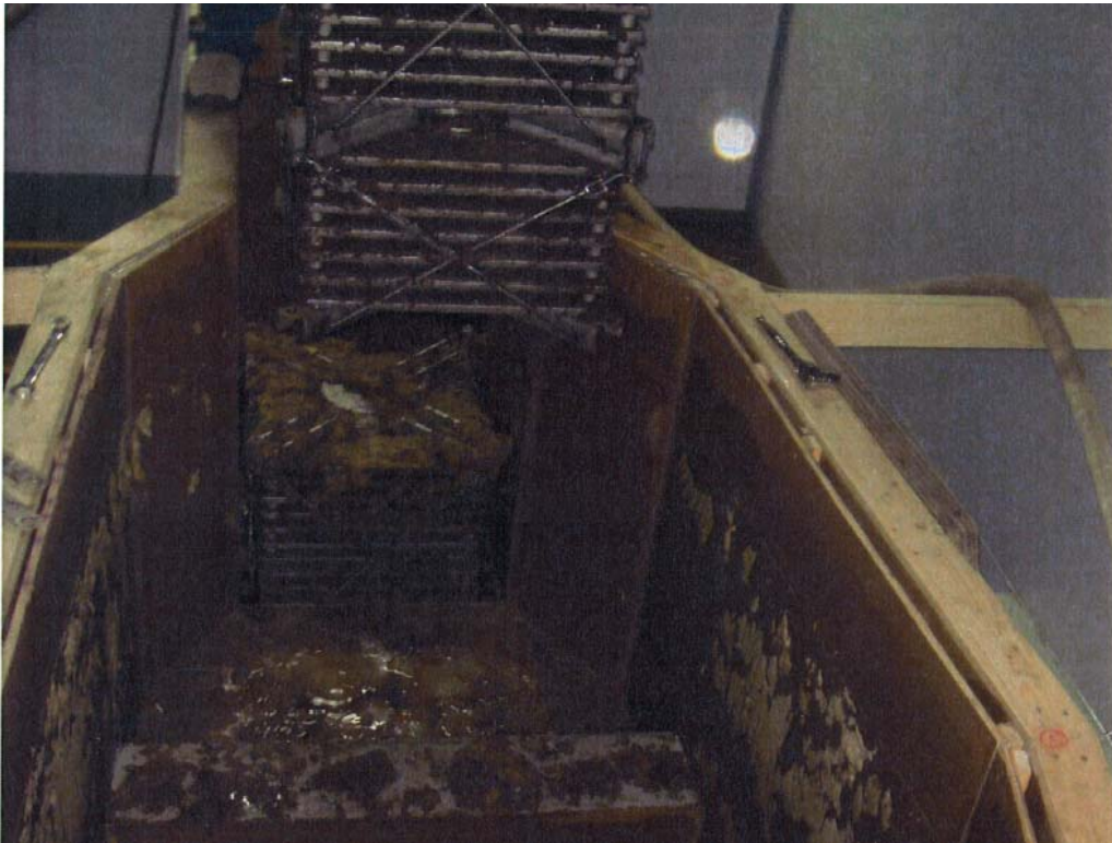
Figure 2. Post Test Debris Accumulation on Top of Strainer Module
