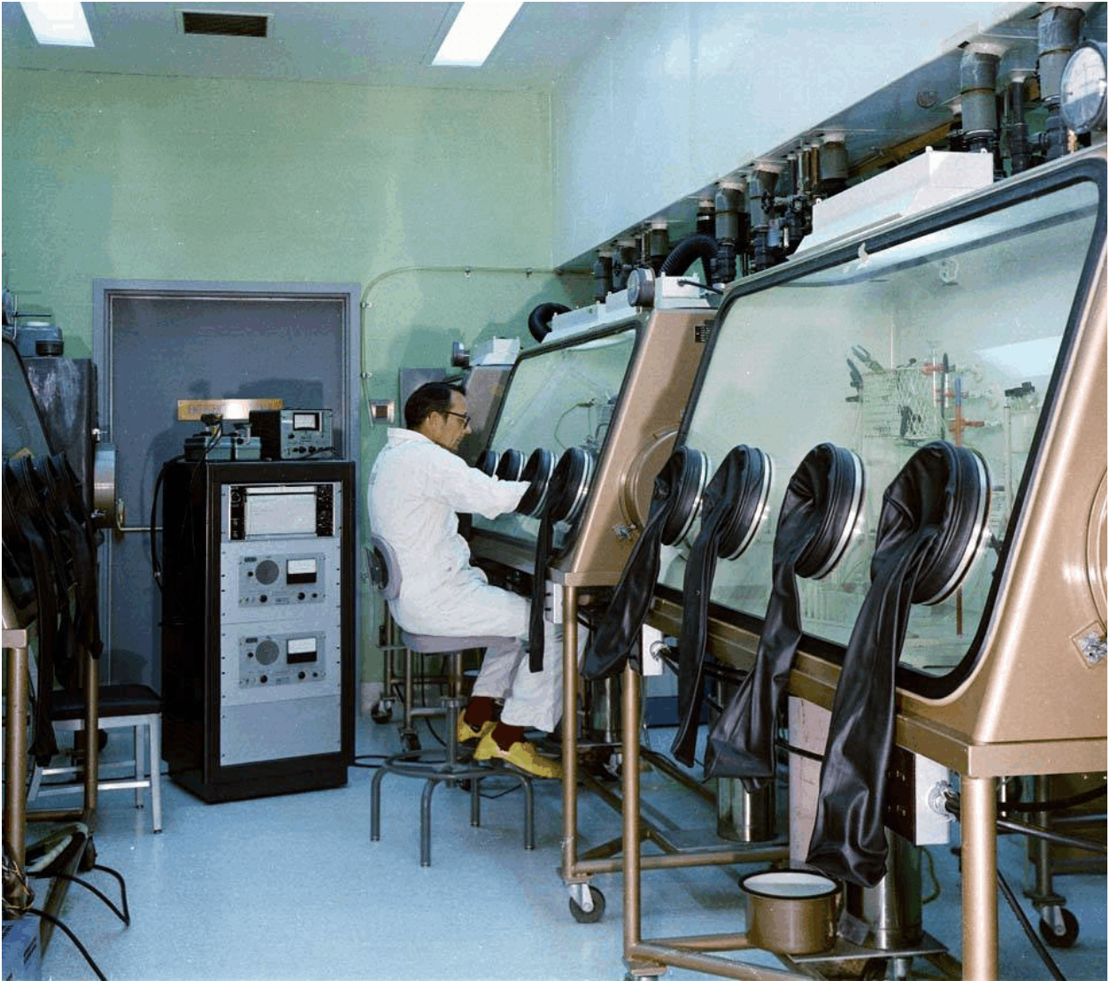
Figure 12: Glove boxes used for handling nuclear materials having low levels of penetrating radiation
