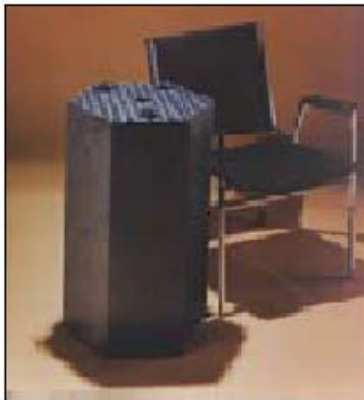
Figure 10: Prismatic HTGR fuel element
