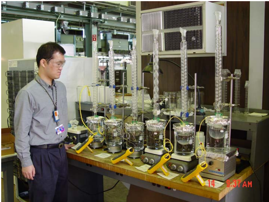
Figure 2. The long-term Al solubility test facility setup.
