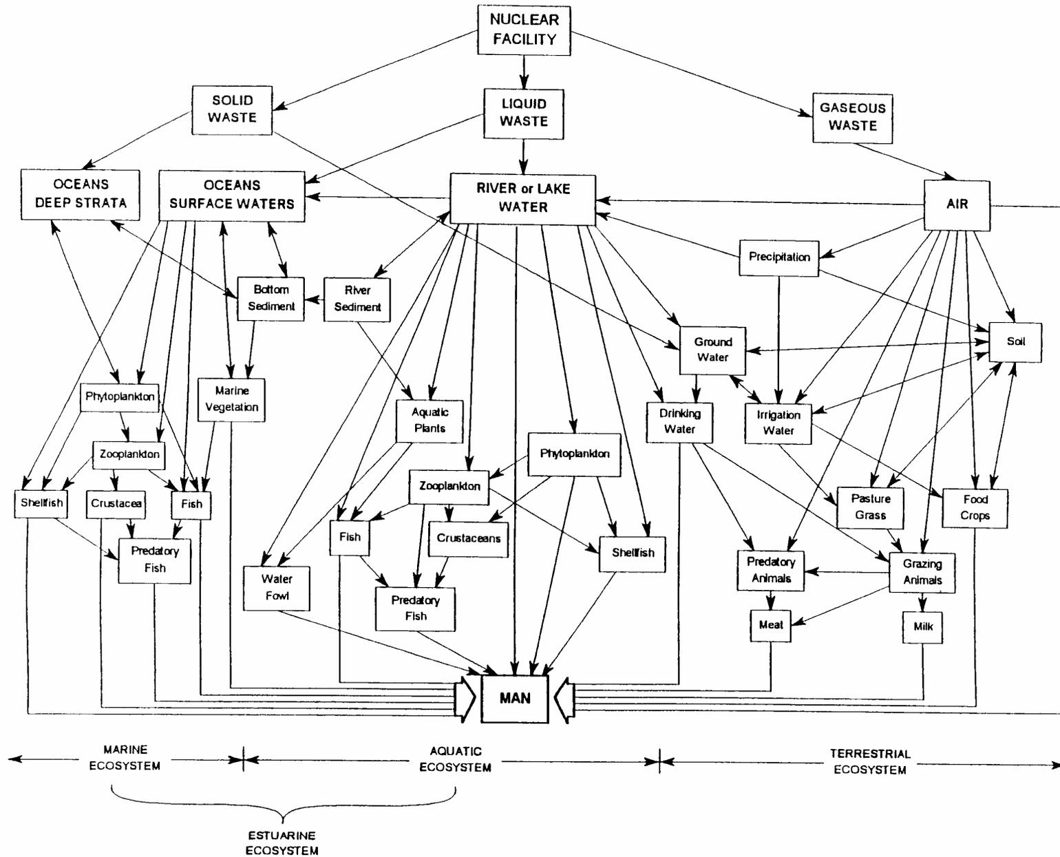
Figure 1. Potential Radiation Exposure Pathways Leading to Man
