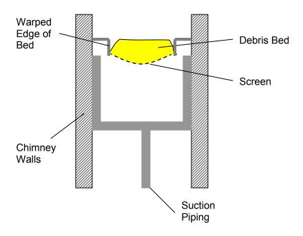
In light of the discussion above, Alion should (a) demonstrate that flow diversion through the thinner debris bed cross section caused by circumferential warping has not had a significant adverse impact on testing conducted at VUEZ and (b) describe measures taken to prevent or minimize this observed phenomenon in future testing.
