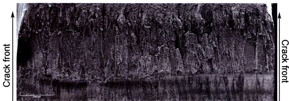
Figure 50. Crack front on fracture surface of sample CT933-TS. Crack advance from bottom to top.
