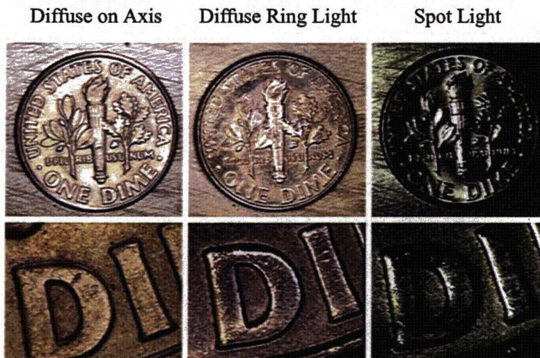
Figure 3.3 Dime Illuminated Using Three Lighting Techniques
