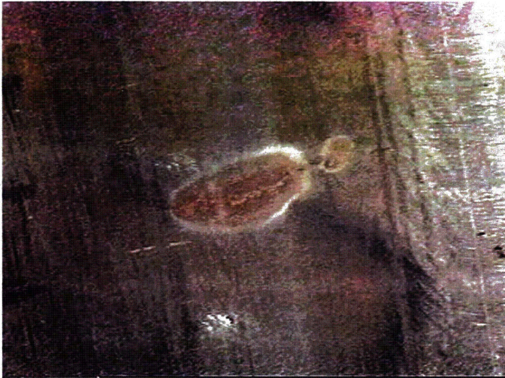
Figure 6.6 Stress Corrosion Crack Through Stainless Steel Made More Visible by Oxide Decoration
