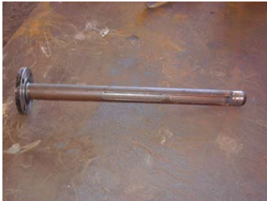
Figure 6 – Photograph illustrating pipe insert that attaches to suction line for air injection into either CA or WDF pump suction line.
