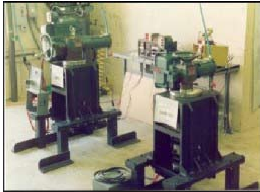
Figure 2 - Cyclic Testing of Limitorque Actuator in Progress
