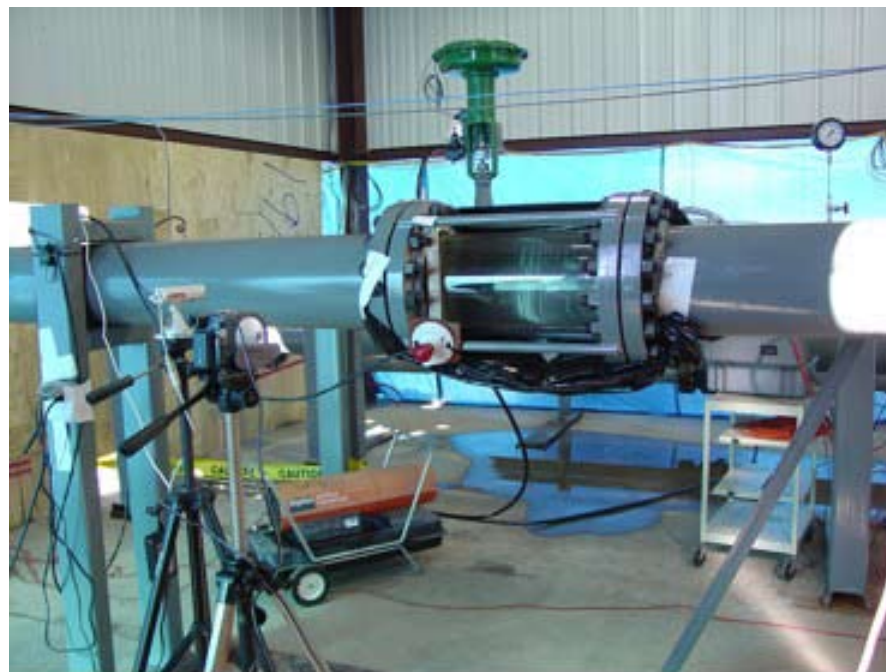
Figure 8 – Photograph illustrating Sight Glass in suction line for CA pump.
