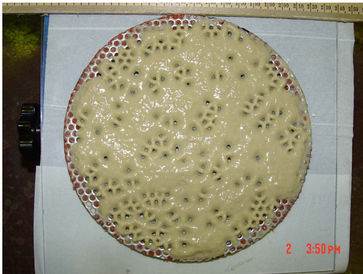
Figure 6. Plan view of debris bed formed by pure CalSil loading (ICET-3-19-A2).
