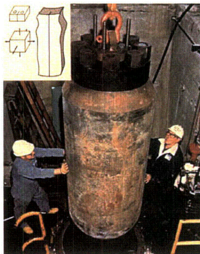
Fig. A-4.2. Test vessel being lowered into outer containment vessel at HSST PTS test facility.
