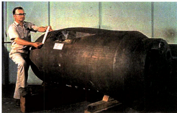
Fig. A-2.4. ITV-6 test vessel was tested under pressure and at a temperature (190°F) well above onset of Charpy upper shelf; fracture was by ductile shear.
