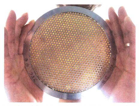
Figure J.16.4. Debris Bed in Test Section After Retrieval, Bottom View.
