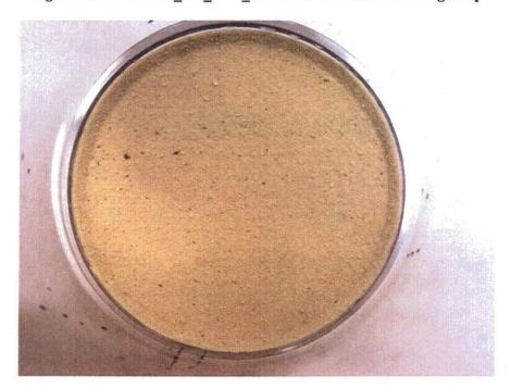
Figure J.12.4. 051117\_NC\_2776\_L1 Debris Bed in Test Section After Retrieval, Top View. Screen pattern is observable on debris bed surface.
