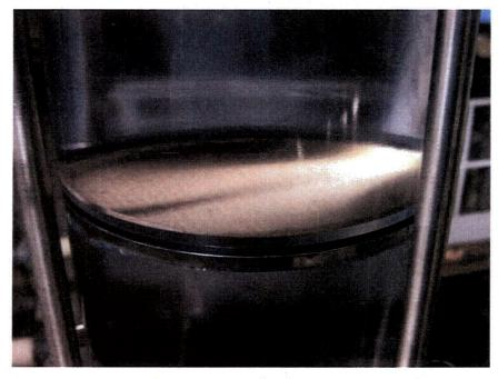
Figure J.7.3. Submerged 051121\_NC\_1586\_L1 Debris Bed During Test. Screen pattern is observable on debris bed surface.
