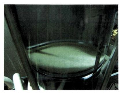
Figure J.11.3. Submerged 051123\_NC\_2181\_L1 Debris Bed During Test. Screen pattern is observable on debris bed surface; flow channel is observable in foreground.
