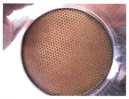
Figure J.5.4. 060426\_NC\_0708\_LP1, LP2 Debris Bed in Test Section After Retrieval, Bottom View
