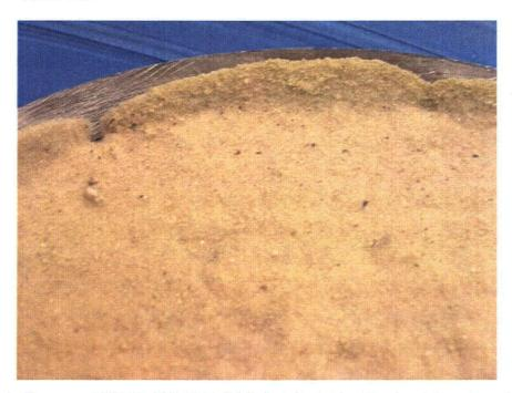
Figure J.11.8. Close-up of 051123\_NC\_2181\_L1 Debris Bed After Retrieval from Test Section.
