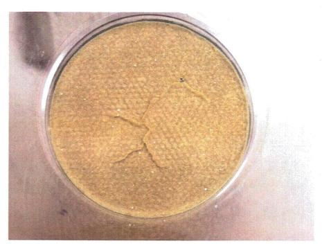
Figure J.4.2. Debris Bed in Test Section After Retrieval, Top View; Disturbed Post-Test
