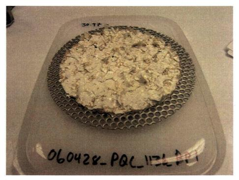
Figure J.2.2. Paint Chip Debris Bed from Test 060428\_PQC\_1136\_BP1 Retrieved from Benchtop Test Loop. The target debris loading was 1.4 kg/m² with a 1 to 1 ratio of 1/4-inch-square to processed material.
