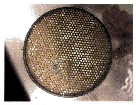
Figure J.1.3. Debris Bed in Test Section After Retrieval, Bottom View; Incomplete Debris Bed
