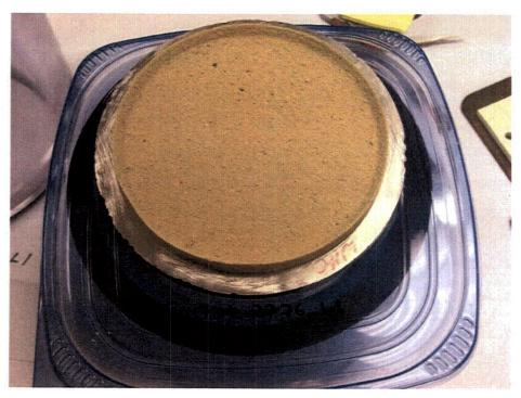
Figure J.12.6. 051117\_NC\_2776\_L1 Debris Bed After Retrieval from Test Section. Screen pattern is observable on debris bed surface.
