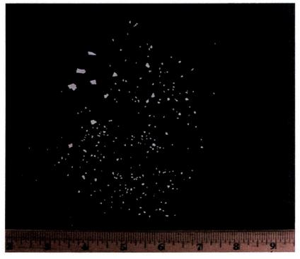
Figure O.1.3. Size Characterization Photo for ZE-Processed Debris. Total mass of particulate in photo was 0.12 g.
