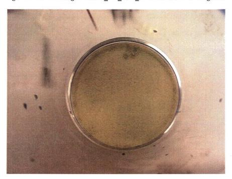
Figure J.9.3. 060331\_NC\_2024\_LP1 Debris Bed in Test Section After Retrieval, Top View. Indentation at approximately 12:30 orientation was the result of water dripping during post-test retrieval.
