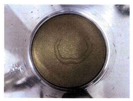
Figure J.15.3. Debris Bed in Test Section After Retrieval, Top View. Disturbed post-test.
