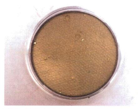
Figure J.16.3. Debris Bed in Test Section After Retrieval, Top View. Disturbed post-test.
