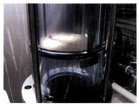
Figure J.12.3. 051117\_NC\_2776\_L1 Debris Bed After Draining Loop
