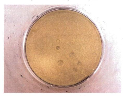
Figure J.17.3. Debris Bed in Test Section After Retrieval, Top View. Disturbed post-test.
