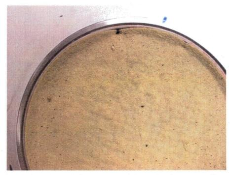
Figure J.11.5. Close-Up of 051123\_NC\_2181\_L1 Debris Bed in Test Section After Retrieval, Top View. Screen pattern is observable on debris bed surface; flow channels are observable at 11:45 and 1:30 orientations.
