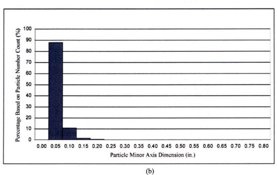
Figure O.1.7. Particle Size Histogram by Number Count for ZE-Processed Debris. Figures a and b are histograms for the major and minor axes, respectively. Distributions obtained from 0.12 g sample presented in Figure O.1.3 and Table O.1.3.
