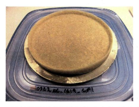
Figure J.8.5. 060323\_NC\_1619\_LP1 Debris Bed After Retrieval from Test Section
