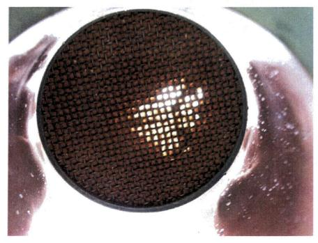
Figure J.3.4. Ruptured 051110\_NC\_0595\_L1 Debris Bed in Test Section After Retrieval, Bottom View; Rupture Caused Post-Test
