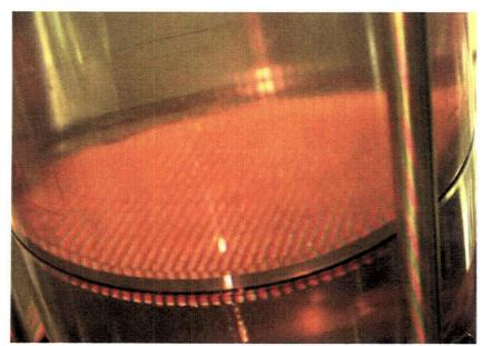
Figure J.6.4. 060517\_NC\_0808\_LP1, LP2 Debris Bed in Test Section During Flow at for Final Test Velocity Phase. Grid lines are from optical triangulation light. Surface irregularities, holes, etc. of Figure J.6.3 are not observable. 11:00 orientation of debris bed in Figure J.41 corresponds to near-left-hand-side of Figure J.42 (note vertical black line on test section above debris bed at described orientation in each photo).
