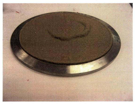
Figure J.15.5. Debris Bed After Retrieval from Test Section. Disturbed post-test.
