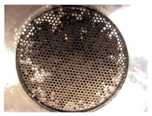
Figure K.1.10. 060504\_PQZ\_2609\_LP1 Debris Bed in Test Section After Retrieval, Bottom View
