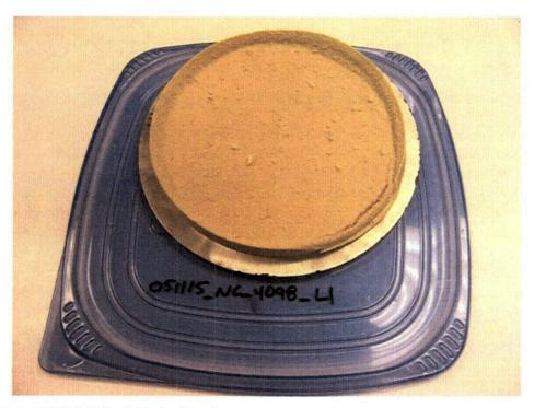
Figure J.14.6. 051115\_NC\_4098\_L1 Debris Bed After Retrieval from Test Section. Collapsed rim was caused following test section retrieval from test loop.
