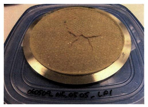
Figure J.4.4. Debris Bed After Retrieval from Test Section; Disturbed Post-Test
