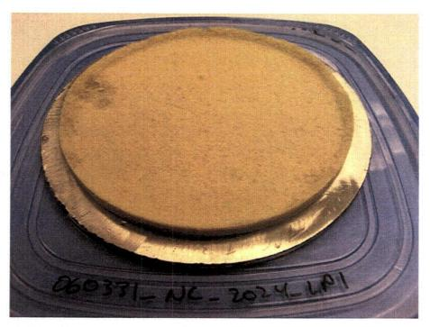
Figure J.9.5. 060331\_NC\_2024\_LP1 Debris Bed After Retrieval from Test Section. Indentation at approximately 9:30 orientation is from water dripping during post-test retrieval.
