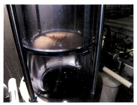
Figure J.3.3. Ruptured 051110\_NC\_0595\_L1 Debris Bed After Draining; Rupture Caused Post-Test
