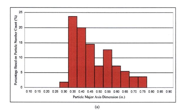
Figure O.1.8. Particle Size Histogram by Number Count for ZE-Chips Debris. Figures a and b are histograms for the major and minor axes, respectively. Distributions obtained from 1 g sample presented in Figure O.1.4 and Table O.1.4.
