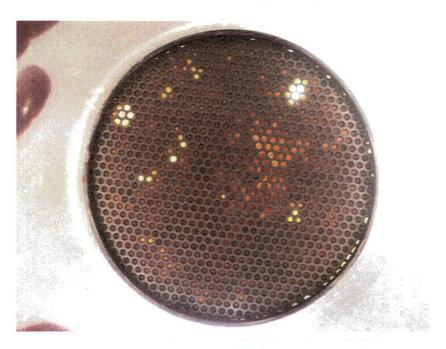
Figure J.6.5. 060517\_NC\_0808\_LP1, LP2 Debris Bed in Test Section After Retrieval, Bottom View. Debris bed disturbed during retrieval (see Figure J.6.3). Some areas of light were visually observed to appear and disappear during testing (see text discussion).
