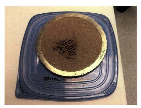
Figure J.3.5. Ruptured 051110\_NC\_0595\_L1 Debris Bed After Retrieval from Test Section; Rupture Caused Post-Test
