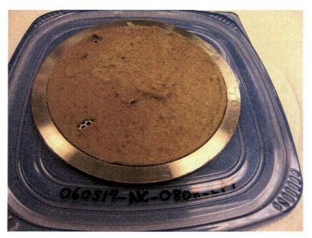
Figure J.6.6. 060517\_NC\_0808\_LP1, LP2 Debris Bed After Retrieval from Test Section. Debris bed disturbed during retrieval (see Figure J.6.3 caption).
