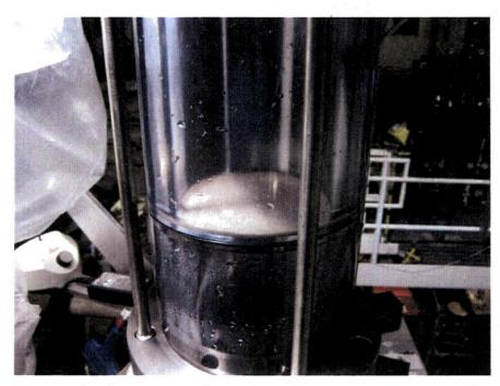
Figure J.10.3. Submerged 060404 NC 2698 LP1 Debris Bed During Test
