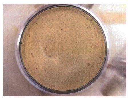
Figure J.7.4. 051121\_NC\_1586\_L1 Debris Bed in Test Section After Retrieval, Top View. Screen pattern is observable on debris bed surface; dark pock-marks are from post-retrieval water drips.
