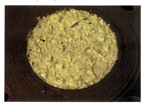
Figure J.2.1. Paint Chip Debris Bed from Test 060428\_PQC\_1136\_BP1 before Removing Debris Bed from Test Section. The target debris loading was 1.4 kg/m² with a 1 to 1 ratio of 1/4-inch-square to processed material.
