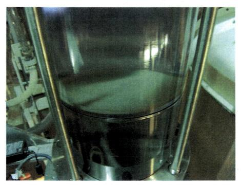
Figure J.9.2. Submerged 060331\_NC\_2024\_LP1 Debris Bed During Test.
