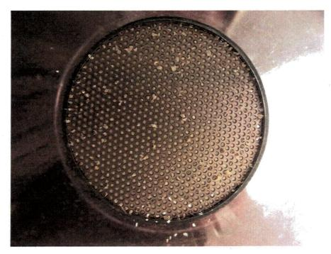
Figure K.1.6. 060501\_PQC\_2609\_LP1, LP2 Debris Bed in Test Section After Retrieval, Bottom View (note penetration of ALK debris into perforations of plate)
