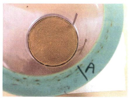
Figure J.5.3. 060426\_NC\_0708\_LP1, LP2 Debris Bed in Test Section After Retrieval, Top View. Debris bed rim separated/rolled in from test section wall by post-retrieval handling.
