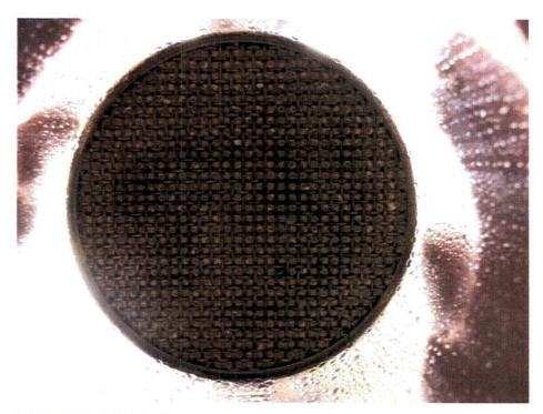
Figure J.12.5. 051117\_NC\_2776\_L1 Debris Bed in Test Section After Retrieval, Bottom View
