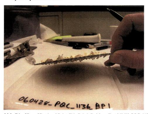
Figure J.2.3. Edge View of Retrieved Paint Chip Debris Bed from Test 060428\_PQC\_1136\_BP1
