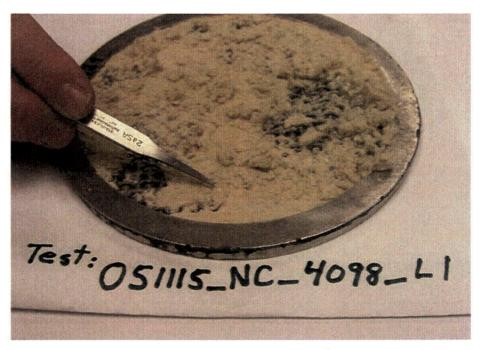
Figure J.14.7. 051115\_NC\_4098\_L1 Debris Bed After Retrieval from Test Section and During Removal From Screen. CalSil particulate is visible throughout debris bed (white particles). Large particle is pointed out.
