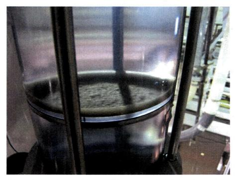
Figure J.8.2. Submerged 060323\_NC\_1619\_LP1 Debris Bed During Test
