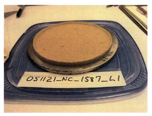
Figure J.7.6. 051121\_NC\_1586\_L1 Debris Bed After Retrieval from Test Section. Screen pattern is observable on debris bed surface.
