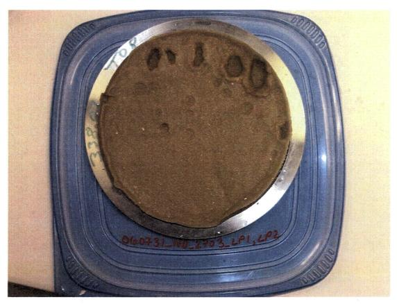
Figure H.6.5. Debris Bed After Retrieval from Test Section, Disturbed Post-Test
