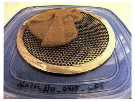
Figure H.1.3. 060321\_NO\_0405\_LP1 Debris Bed After Retrieval. The disturbance consisted of the entire debris bed floating up under severely reduced flow conditions, flipping over and folding up, and then re-depositing on the plate once flow was increased. The debris bed was visually observed to remain essentially intact.
