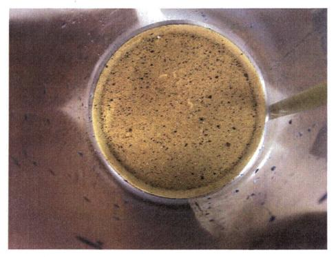
Figure H.4.4. 051108\_NO\_3067\_L1 Debris Bed in Test Section After Retrieval, Top View
