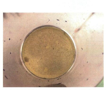
Figure H.2.2. 060313\_NO\_1349\_LP1 Debris Bed in Test Section After Retrieval, Top View
