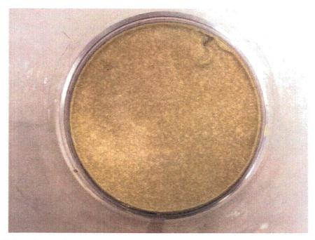
Figure H.7.3. Debris Bed in Test Section After Retrieval, Top View. Disturbed post-test.
