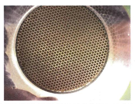
Figure H.3.5. 060425\_NO\_2703\_LP1, LP2, LP3 Debris Bed in Test Section After Retrieval, Bottom View
