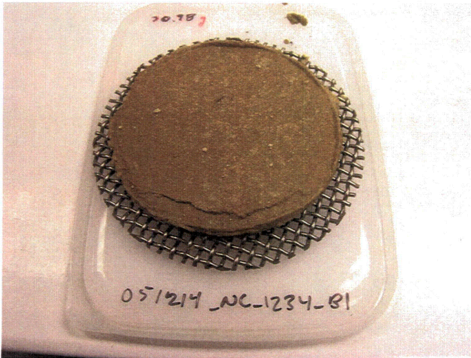
Figure 6.17. Test 051214_NC_1234_B1 NUKON/CalSil Debris Bed for Case 1A. Debris Bed Surface is Mostly CalSil.
