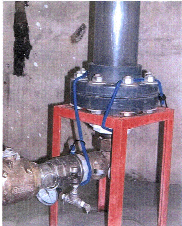
Figure 2.5. Downstream Portion of Benchtop Test Section Showing Pressure Tap Location
