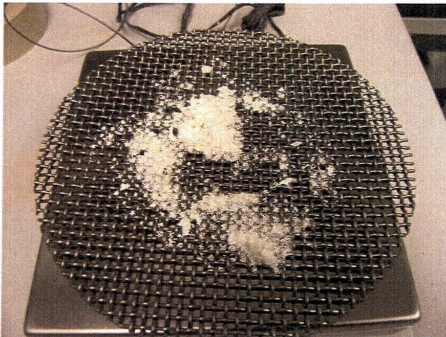
Figure 4.3. ALK Debris Poured onto 5-Mesh Screen for R4 Evaluation, R4 ~ 1.4
