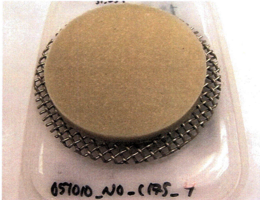
Figure 3.27. Example NUKON Debris Bed for R4D2 (target debris loading of 1449.5 \text{ g/m}^2 )
