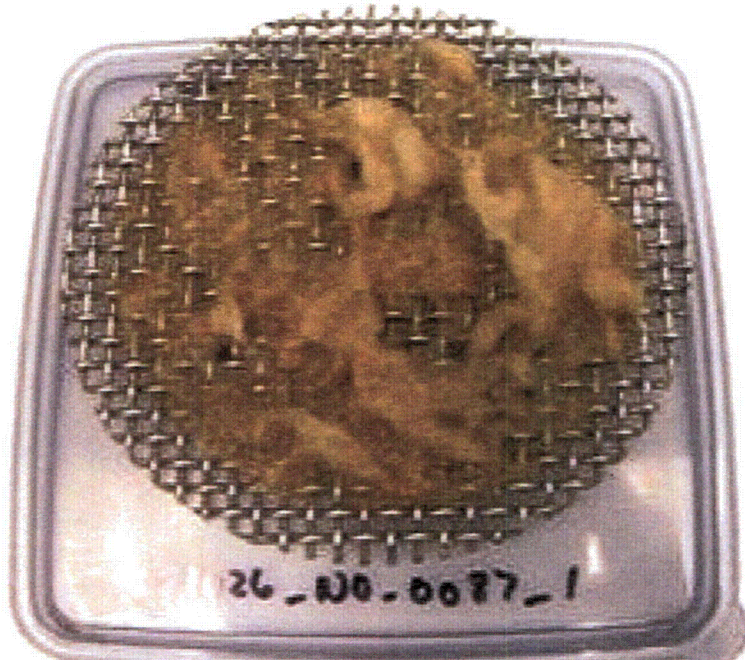
Figure 3.11. NUKON Debris Bed for 107.3 \text{ g/m}^2 Target Debris Loading (R4 ~ 20, no blender preparation)
