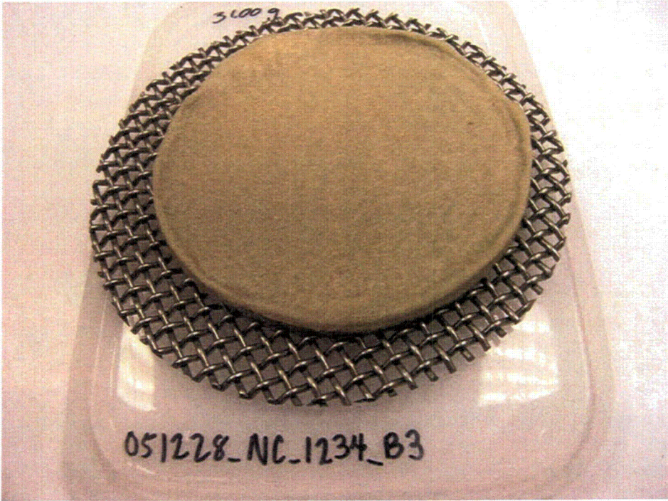
Figure 6.22. Test 051228_NC_1234_B3 NUKON/CalSil Debris Bed for Case 4C
