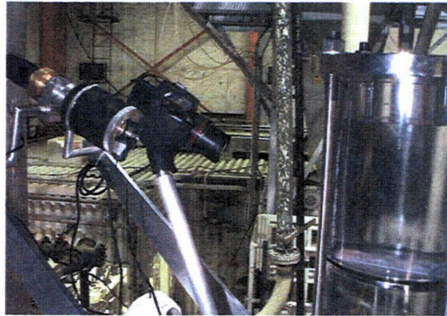
Figure 2.11. Photos of Optical Triangulation System Installed on the Large-Scale Test Loop
