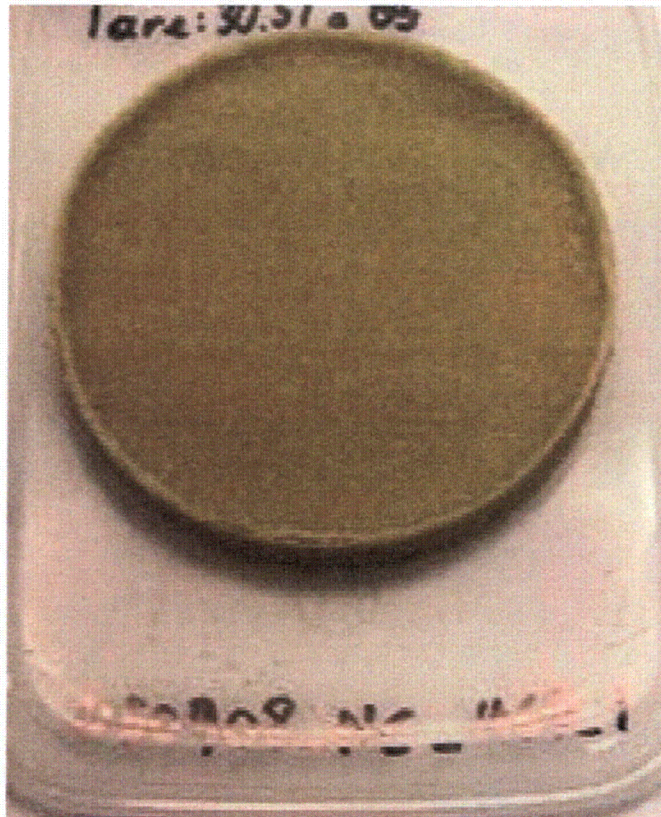
Figure 3.16. NUKON and CalSil Debris Bed for 1811.9 g/m 2 Target Debris Loading (NUKON R4 ~ 11, CalSil R4 < 1 = 1.55) (see Section 3.2.2)
