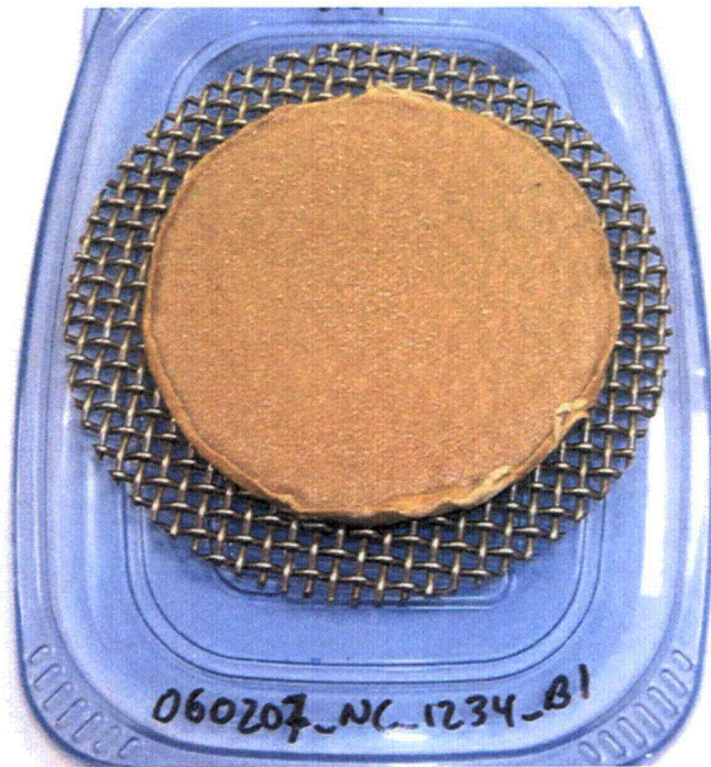
Figure 6.25. 060207_NC_1234_B1 NUKON/CalSil Debris Bed for Case 4 30 sec Lag Time
