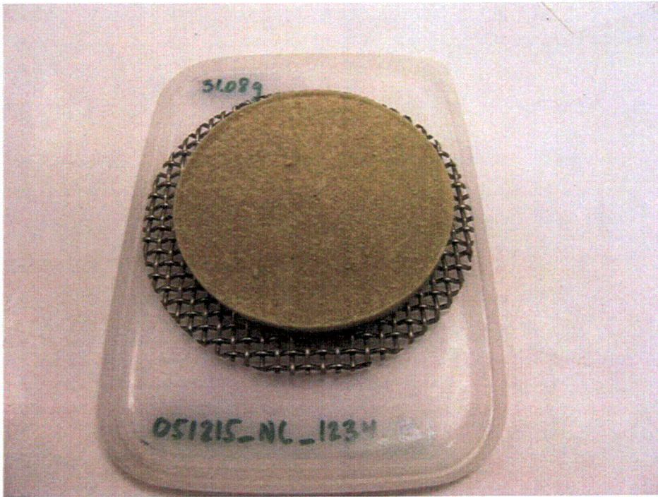
Figure 6.21. Test 051215_NC_1234_B1 NUKON/CalSil Debris Bed for Case 2A.
