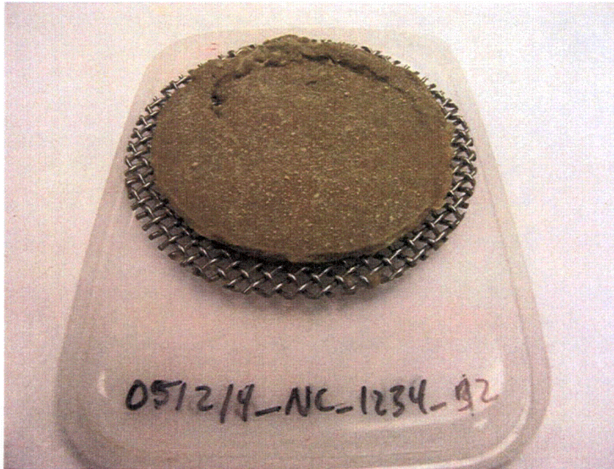
Figure 6.19. Test 051214_NC_1234_B2 NUKON/CalSil Debris Bed for Case 1B. Debris Bed Surface is CalSil. Apparent Post-Test Rupture Caused After Drainage of the Test Loop During Separation of Test Section.
