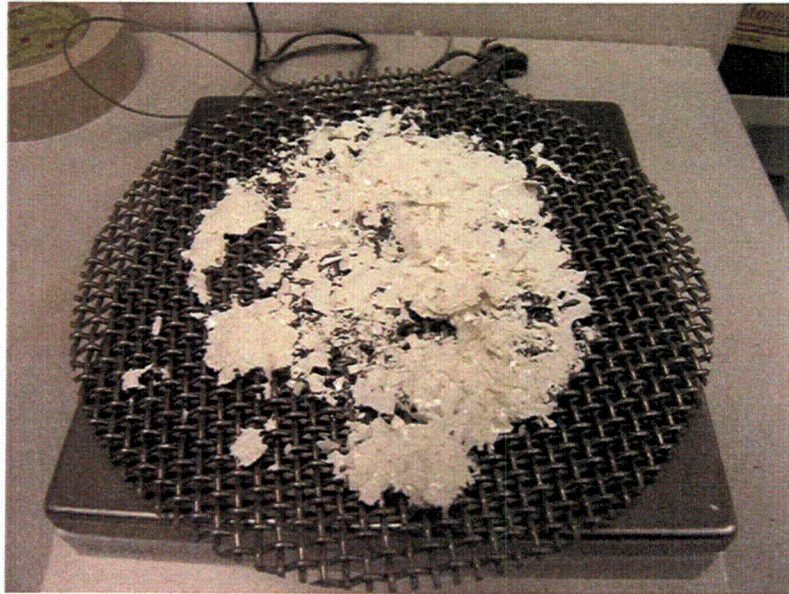
Figure 4.1. ALK Debris Poured onto 5-Mesh Screen for R4 Evaluation, R4 ~ 3.3
