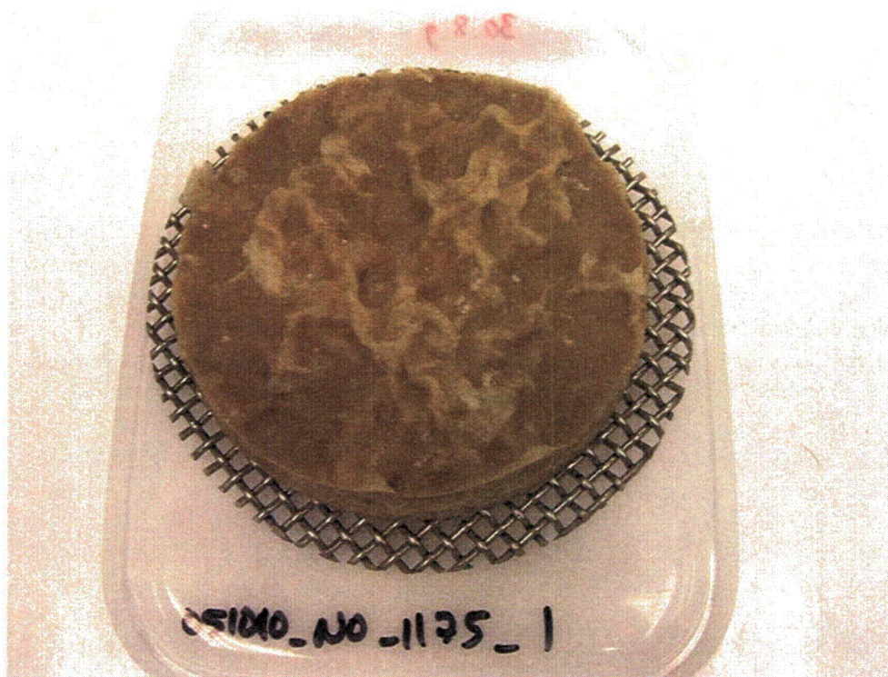
Figure 3.25. Example NUKON Debris Bed for R4A (target debris loading of 1449.5 \text{ g/m}^2 )
