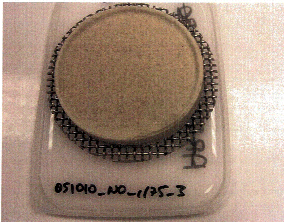
Figure 3.26. Example NUKON Debris Bed for R4C (target debris loading of 1449.5 \text{ g/m}^2 )
