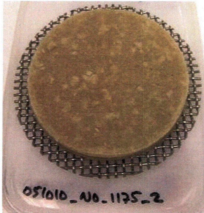
Figure 3.10. NUKON Debris Bed for 1449.5 \text{ g/m}^2 Target Debris Loading (R4 ~ 16)
