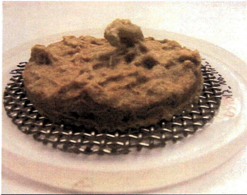
Figure 3.9. NUKON Debris Bed for 1449.5 \text{ g/m}^2 Target Debris Loading (R4 ~ 17 as-received material/no blender preparation)
