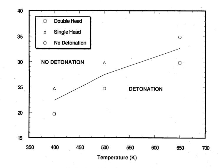
Figure 3.22: Detonability limit for stoichiometric hydrogen-air and steam at 0.1 MPa in the SSDA
