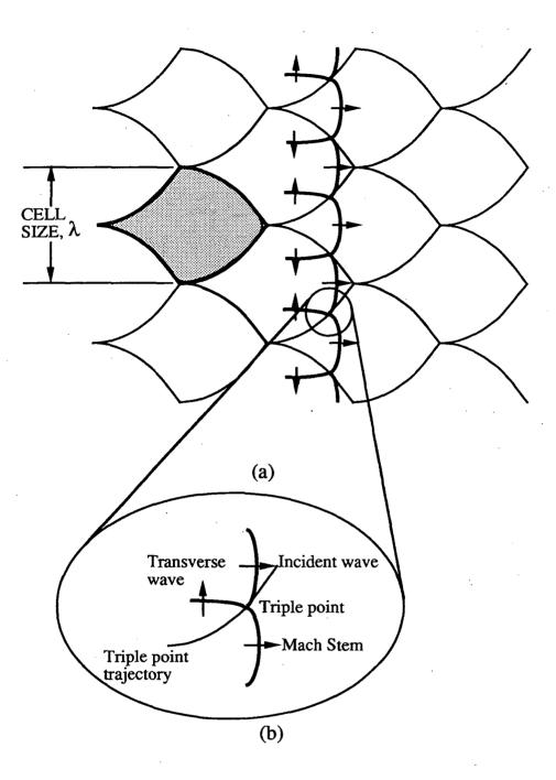
Figure 1.2: (a) Cellular structure of a detonation front and the "fish scale" pattern produced by the triple point trajectories; (b) inset from (a), showing the labelling convention for a three wave interaction
