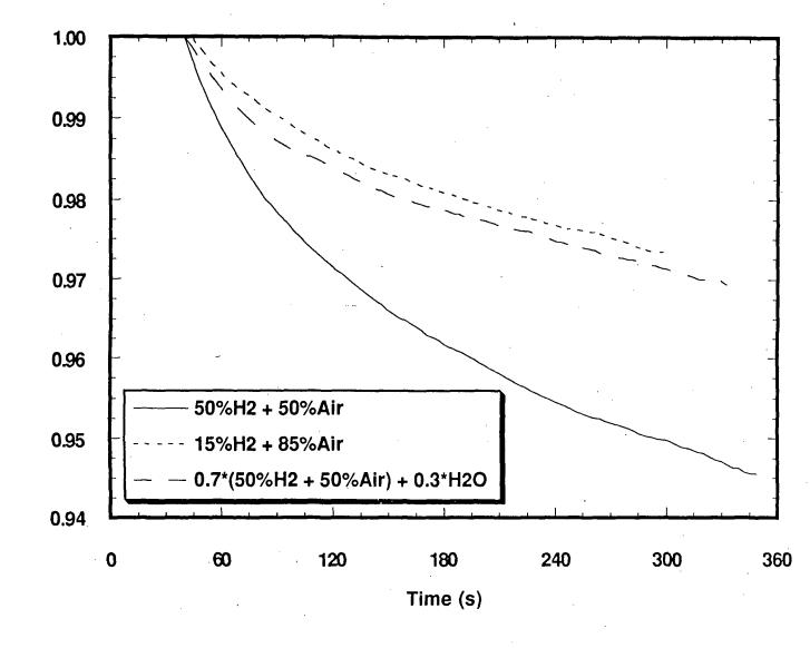
Figure 3.3: Test vessel pressure during slow oxidation of hydrogen-air-steam mixtures at 650K
