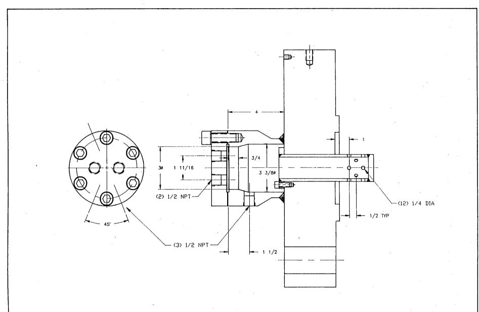
Figure A.2 Mechanical Drawing of Gas Driver Endcover Including Initiation Chamber
