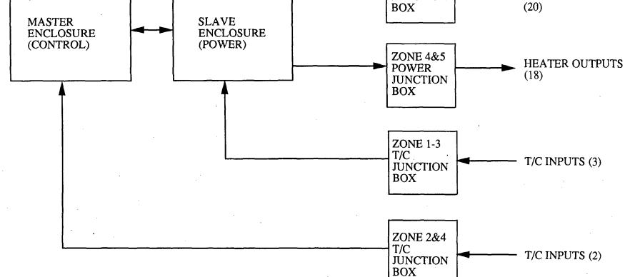
Figure 2.8: Heating system configuration diagram
