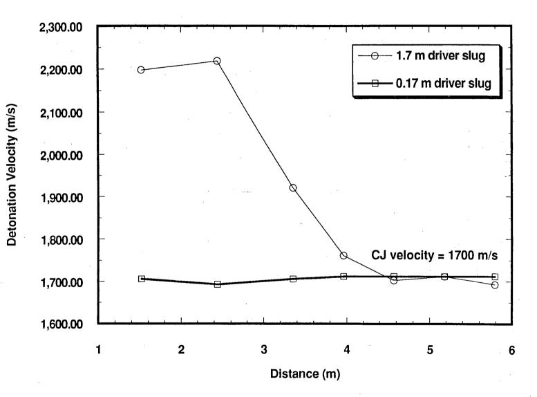
Figure 3.14: Effect of driver slug length on detonation velocity in a 20% hydrogen and 80% air mixture at 300K and 0.1 MPa
