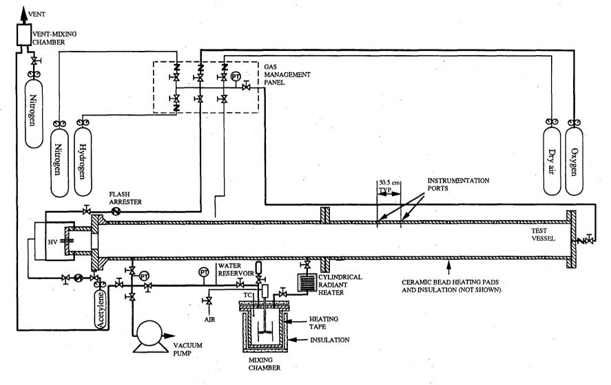
Figure 2.3: Schematic of SSDA showing the test vessel, mixing chamber and secondary piping
