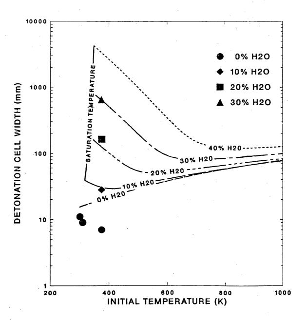
Figure 1.3: The effect of initial temperature on the detonation cell width as a function of steam dilution for stoichiometric hydrogen-air-steam mixture at 1 atm initial pressure (Stamps et al., 1991).
