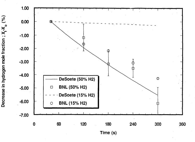
Figure 3.5: Comparison of slow oxidation SSDA grab sample results of Hydrogen-Air at 650K with prediction from Equation (3-2)
