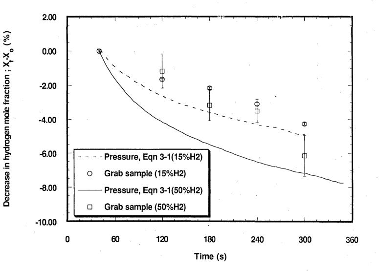
Figure 3.4: Comparison of hydrogen depletion results for slow oxidation of hydrogen-air at 650K using grab samples and inferring from test vessel pressure history using Equation (3-1)
