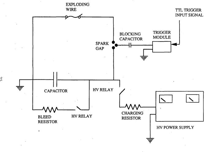
Figure 2.7: High voltage discharge circuit used for initiation in the driver ststem
