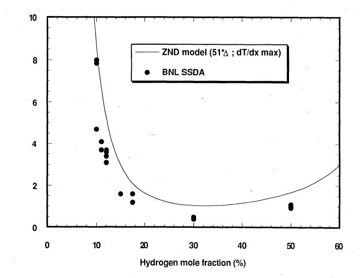
Figure 3.10: Comparison of the measured average detonation cell size and the ZND model prediction for hydrogen-air at 650K and 0.1 MPa
