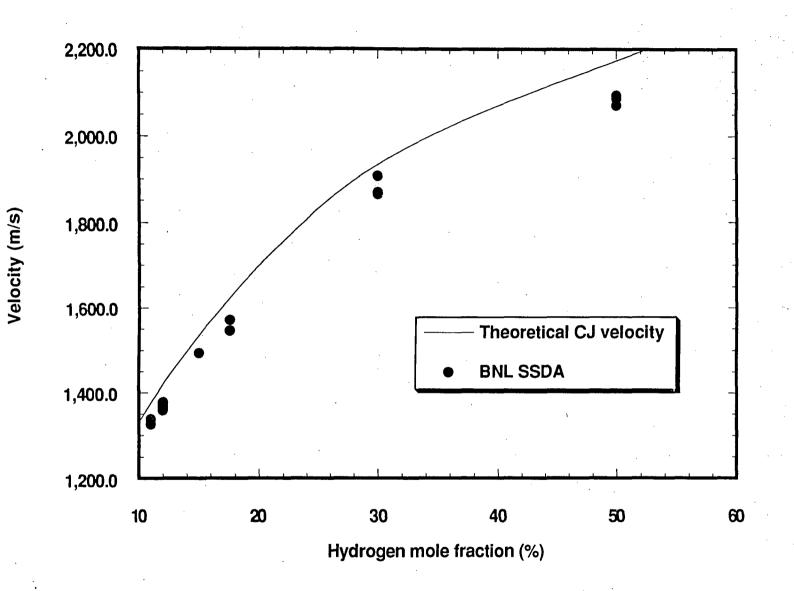
Figure 3.17: Comparison of experimentally measured detonation velocity for hydrogen-air mixtures at 650K with the theoretical CJ velocity
