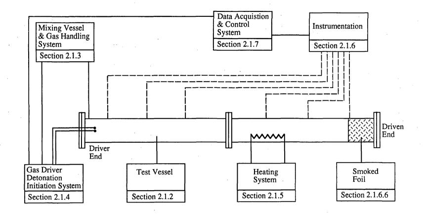
Figure 2.1 Schematic overview of test vessel and operating system
