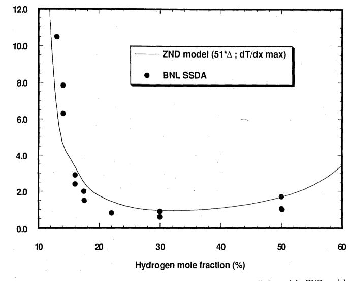
Figure 3.9: Comparison of the measured average detonation cell size and the ZND model prediction for hydrogen-air at 500K and 0.1 MPa
