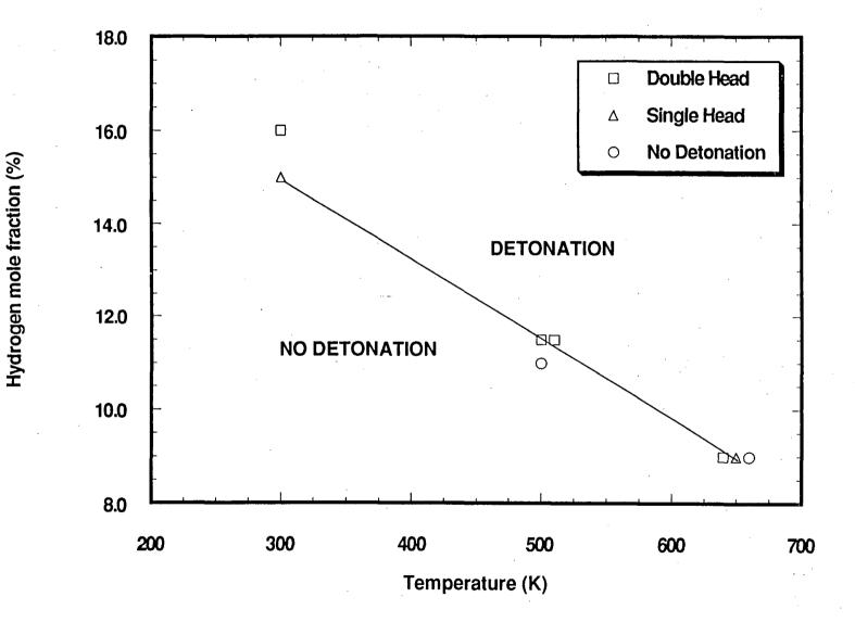
Figure 3.20: Detonability limit for hydrogen-air mixtures at 0.1 MPa in the SSDA
