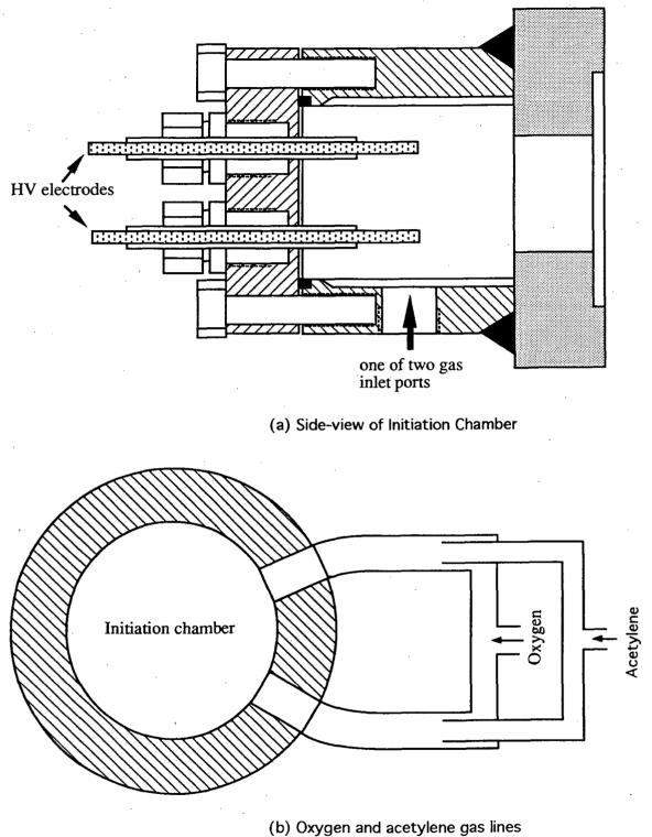
Figure 2.5: Schematic of the Gas Driver System
