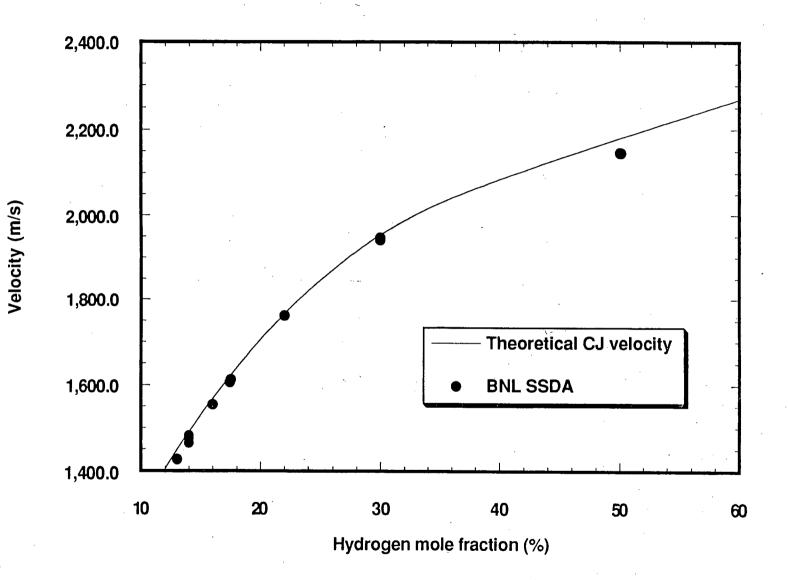
Figure 3.16: Comparison of experimentally measured detonation velocity for hydrogen-air mixtures at 500K with the theoretical CJ velocity
