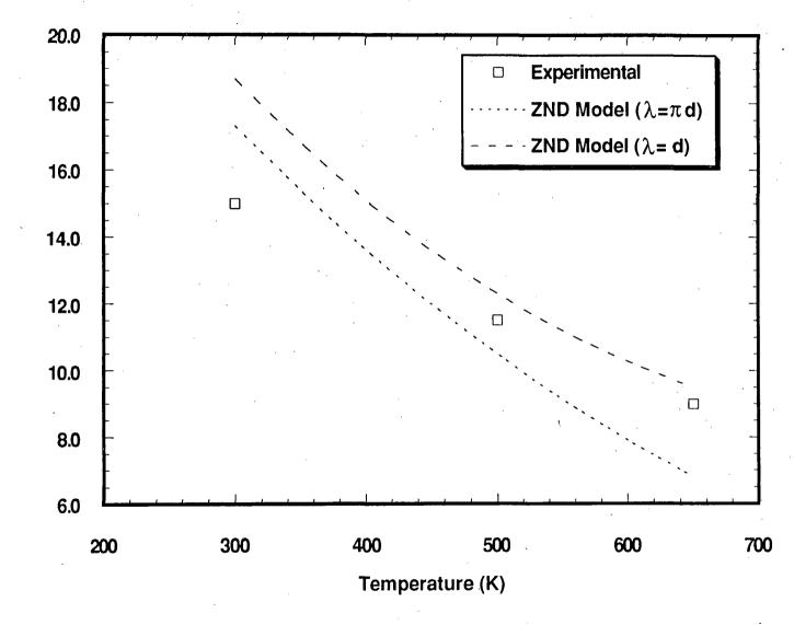
Figure 3.21: Comparison of SSDA experimentally determined detonability limit with ZND model predictions for hydrogen-air mixtures at 0.1 MPa
