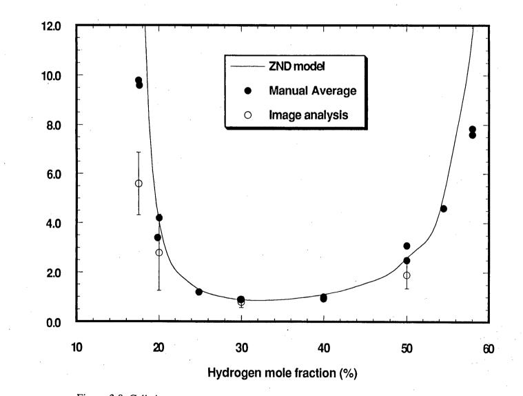
Figure 3.8: Cell size measurement using image analysis overlayed on the data from Figure 3.7
