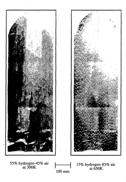
Figure 1.1: Smoked foil records obtained from the SSDA for detonations in hydrogen-air mixtures at 0.1 MPa
