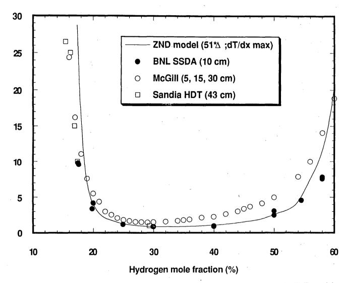
Figure 3.7: Comparison of the measured average detonation cell size and the ZND model prediction for hydrogen-air at 300K and 0.1 MPa
