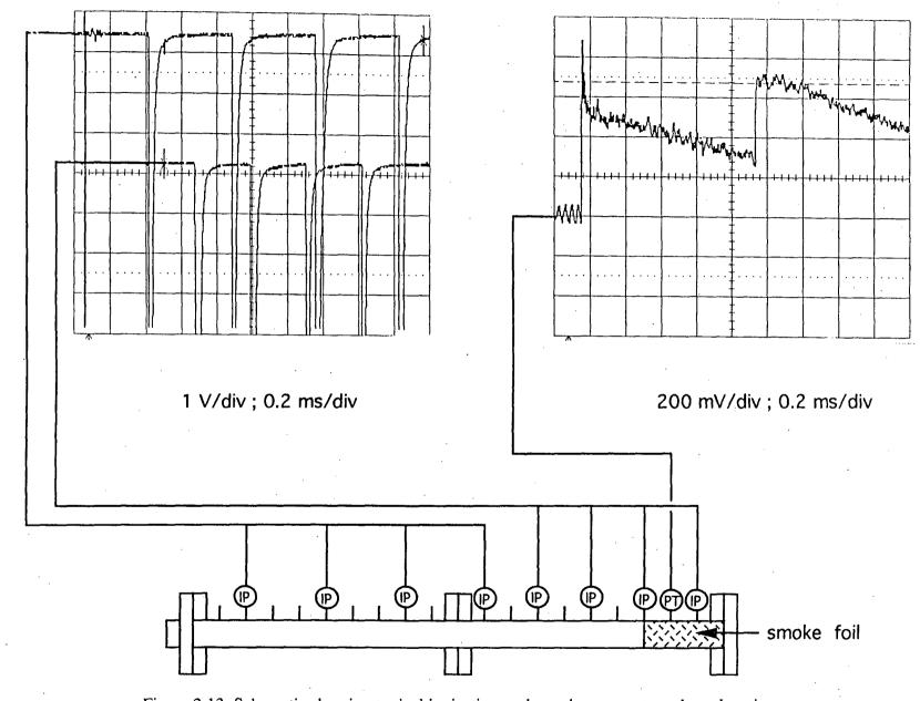
Figure 2.13: Schematic showing typical ionization probe and pressure transducer locations on the test vessel and output signals as recorded on the oscilloscope
