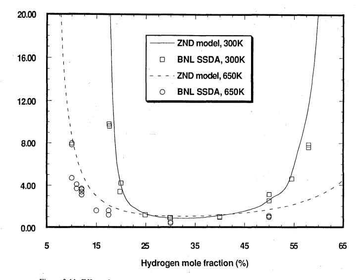
Figure 3.11: Effect of temperature on the average detonation cell size for hydrogen-air mixtures
