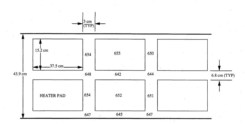
Figure 2.11: Temperature distribution on outer surface of test vessel at 650K (all temperatures in degrees K)
