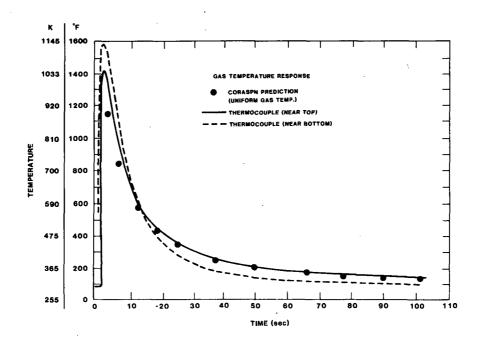
Figure 4-1. Gas Temperature Response Resulting From a 15% Hydrogen Burn in VGES - Predicted vs. Thermocouple Measurements.
