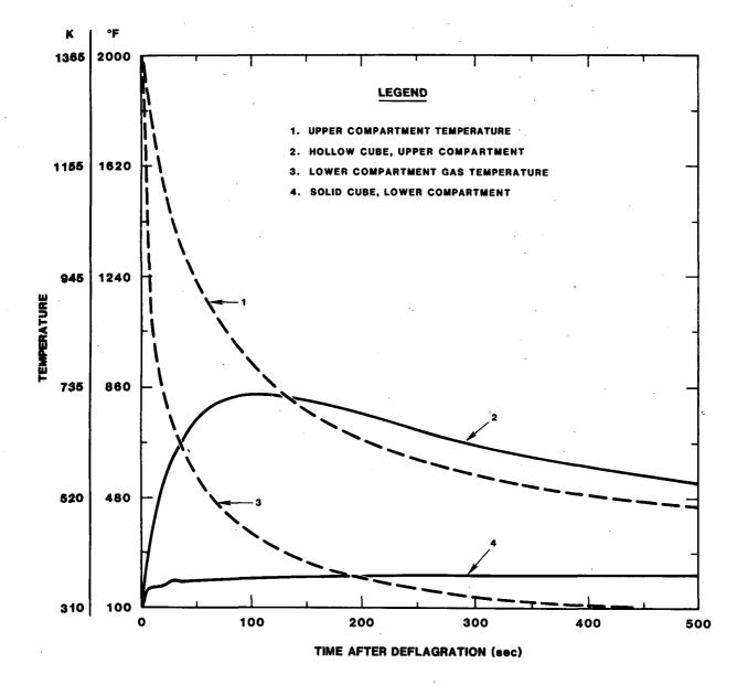
Figure 5-3. Predicted Sequoyah Gas and Hypothetical Component Profiles Resulting From a 10% Hydrogen Burn in the Sequoyah Containment
