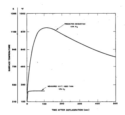
Figure 5-2. Comparison of Hollow Aluminum Cube Thermal Response Obtained From VGES Experiments and Sequoyah Upper Compartment Analysis
