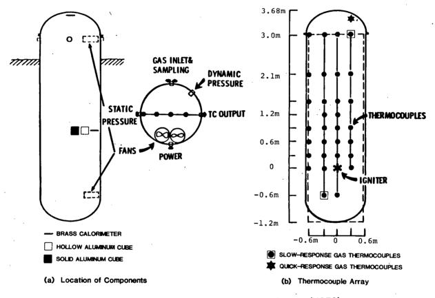
Figure 2-1. Variable Geometry Experimental System (VGES)
