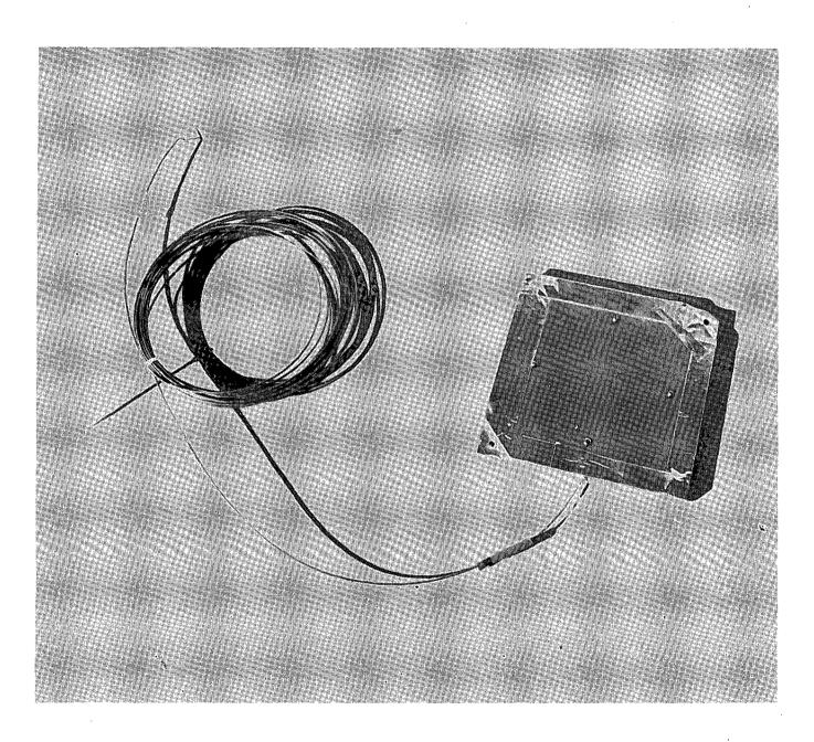
Figure 2-2. Flat-Plate Calorimeter
