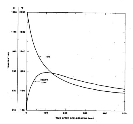
Figure 3-3. Temperature Profiles of Gas and Hollow Aluminum Cube Resulting From a 10% Hydrogen Burn in the Sequeyah Lower Compartment
