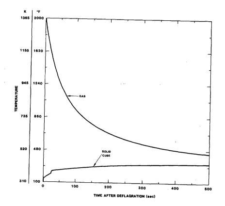
Figure 3-4. Temperature Profiles Gas and Solid Aluminum Cube Resulting From a 10 % Hydrogen Burn in the Sequoyah Upper Compartment
