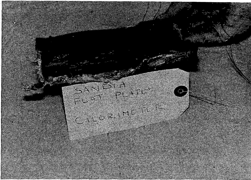
Figure 23: Photograph of brass flat-plate calorimeter, taken after testing
