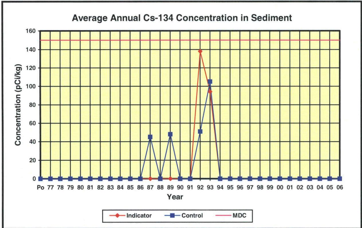
The positive results for Cs-134 appear mostly at the control station. Due to its relatively short half-life of approximately 2 years, the positive results may be attributed to the Chernobyl incident. The overall plotting of the positive results does not show any discernible trends.
