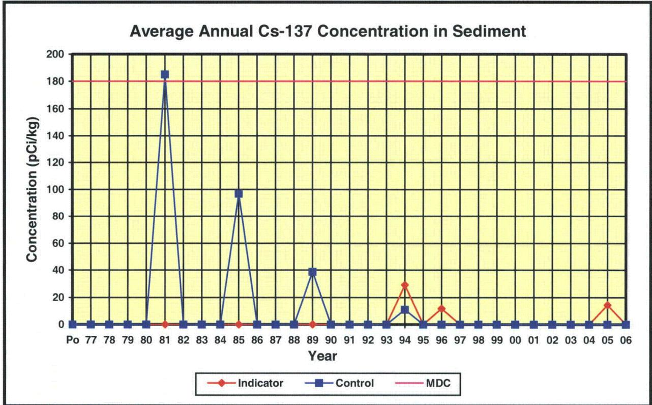
Cs-137 appears to be trending down since the ceasing of above ground weapons testing and the majority of the positive results appear at the control stations. Therefore in general, the positive results can be attributed to the weapons tests and the Chernobyl incident.
