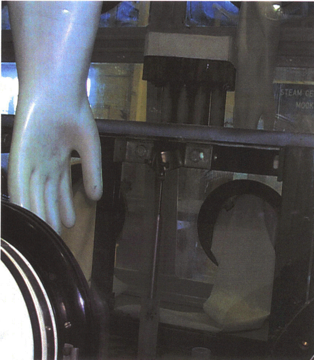
Figure 3.2 Photograph of section of the retired SG tube sheet placed in the Argonne NDE Glove Box. The tube sheet section (seen at top center of photo) contains 12 tubes and is ready for eddy current examination. Each tube extends 7.5 cm above and below the roll transition. The eddy current probe enters the tube from below.
