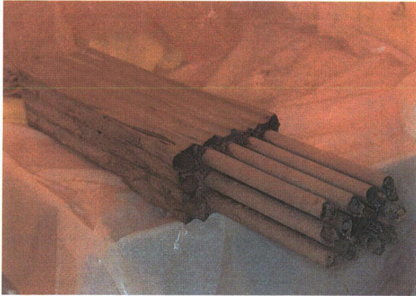
Figure 3.16 Tube sheet section TS1 removed from steam generator D (SGD) (4x3 array of 19-mm (3/4-in.) tubes).
