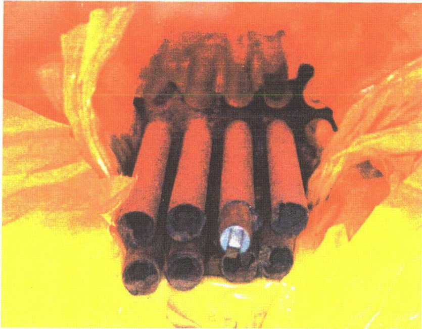
Figure 3.17 Tube sheet section TS2 removed from SGD (4x2 array of 19-mm (3/4-in.) diameter tubes).
