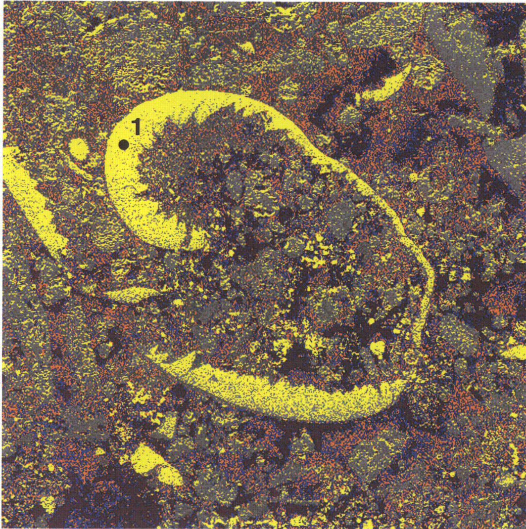
Figure 3.34 SEM image of cross section parallel to tube axis near maximum EC signals in deposit. Sample R39 C45 (ANL 8) at 100X. EDS analysis showed Fe 69.3, Cr 20.0, and Ni 10.7 (in wt. %).
