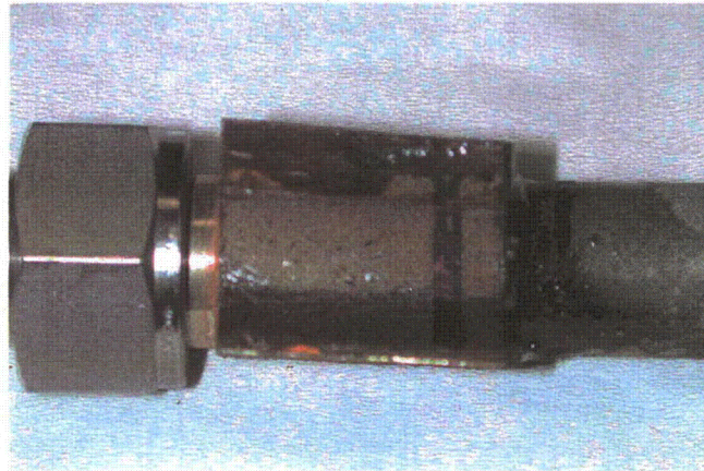
Figure 3.5 Photograph of Alloy 600, 19.1-mm (3/4-in.) diameter, test section #8 from retired steam generator after pressure testing. Some tube sheet material remains around the tube after reducing its size for pressure testing. Fittings to carry out the pressure test are attached to the ends of the tube. The top of the TS is on the right side of the photograph at the end of the tube.
