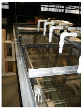
Figure 4 View of ARL test tank with PI prototype strainer installed
