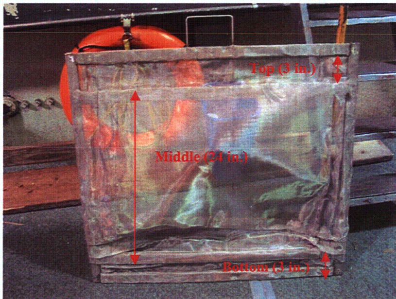
Figure 4-5 Filter for Transport Flume
