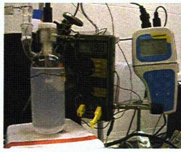
Figure C14. NaAlO 2 solution at 19.8°C. Cooling time 17-h. pH decreased to 9.46 (may be due to CO 2 ).
