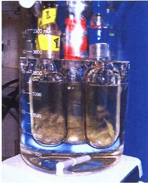
Figure E3. NUKON (2-g/l ratio) exposed in three different solutions; TSP (left), NaOH (middle), and STB (right) at 60°C.
