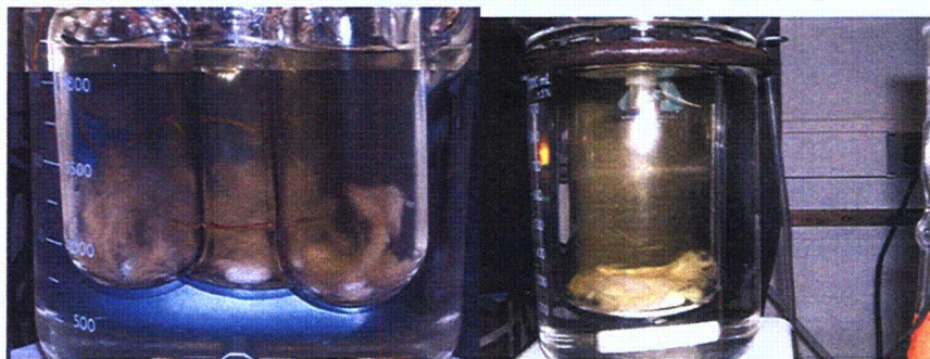
Figure E6. The NUKON enforced settled 40-min ago for popping up the bubbles by glass rod to learn the bubble formation profile in this period of exposure. Time = 167.58-h, T = 60°C. For the Al/NaOH, NUKON settled down from the beginning. Time = 97.08-h, T = 60°C
