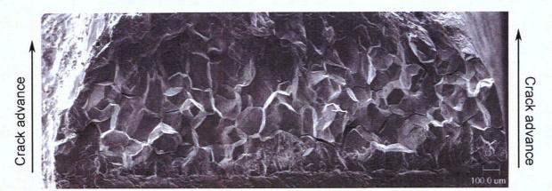
Figure 42. Micrograph of the fracture surface of Specimen N3CC-2. Crack advance is from bottom to top.
