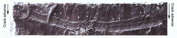
Figure 48. Crack front on Sample J11CC-1. Crack growth is from top to bottom.
