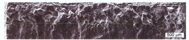
Figure 39. Micrograph of the fracture surface of Specimen N3CL-1. Crack advance is from top to bottom.
