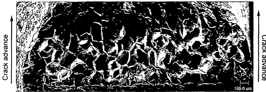
Figure 47. Micrograph of the fracture surface of Specimen N3CC-2. Crack advance from bottom to top.
