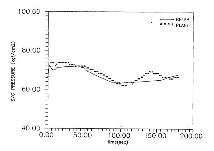
Figure 5.7 STEAM GENERATOR PRESSURE
