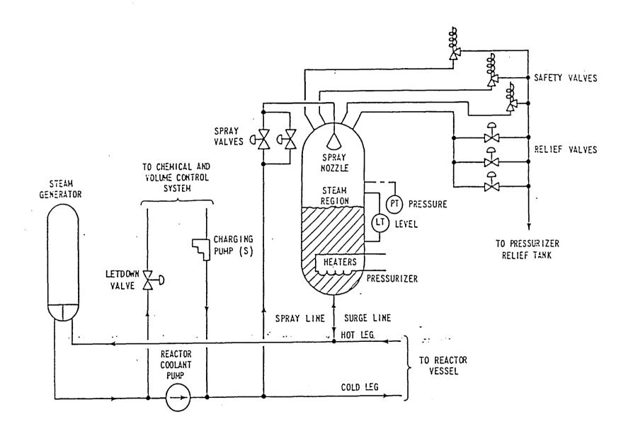
Figure 2-2 Pressurizer Pressure and Level Associated Equipment Arrangement
