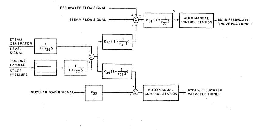
Figure 2-5 Functional Block Diagram of the Steam Generator Level Control System
