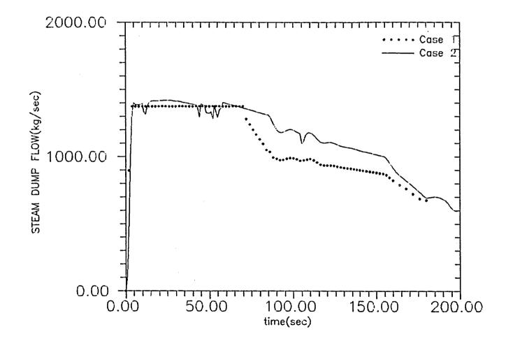
Fig. 7.2 Nodalization study (steam dump flow)
