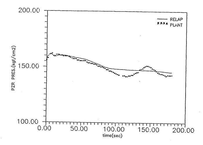
Figure 5.4 PRESSURIZER PRESSURE
