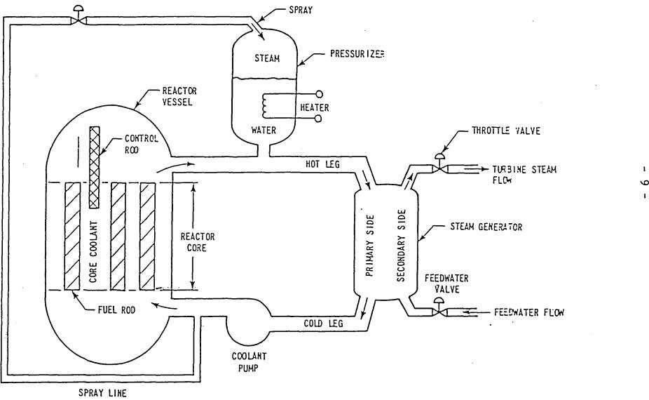
Figure 2-1. Pressurized Water Reactor Schematic Diagram
