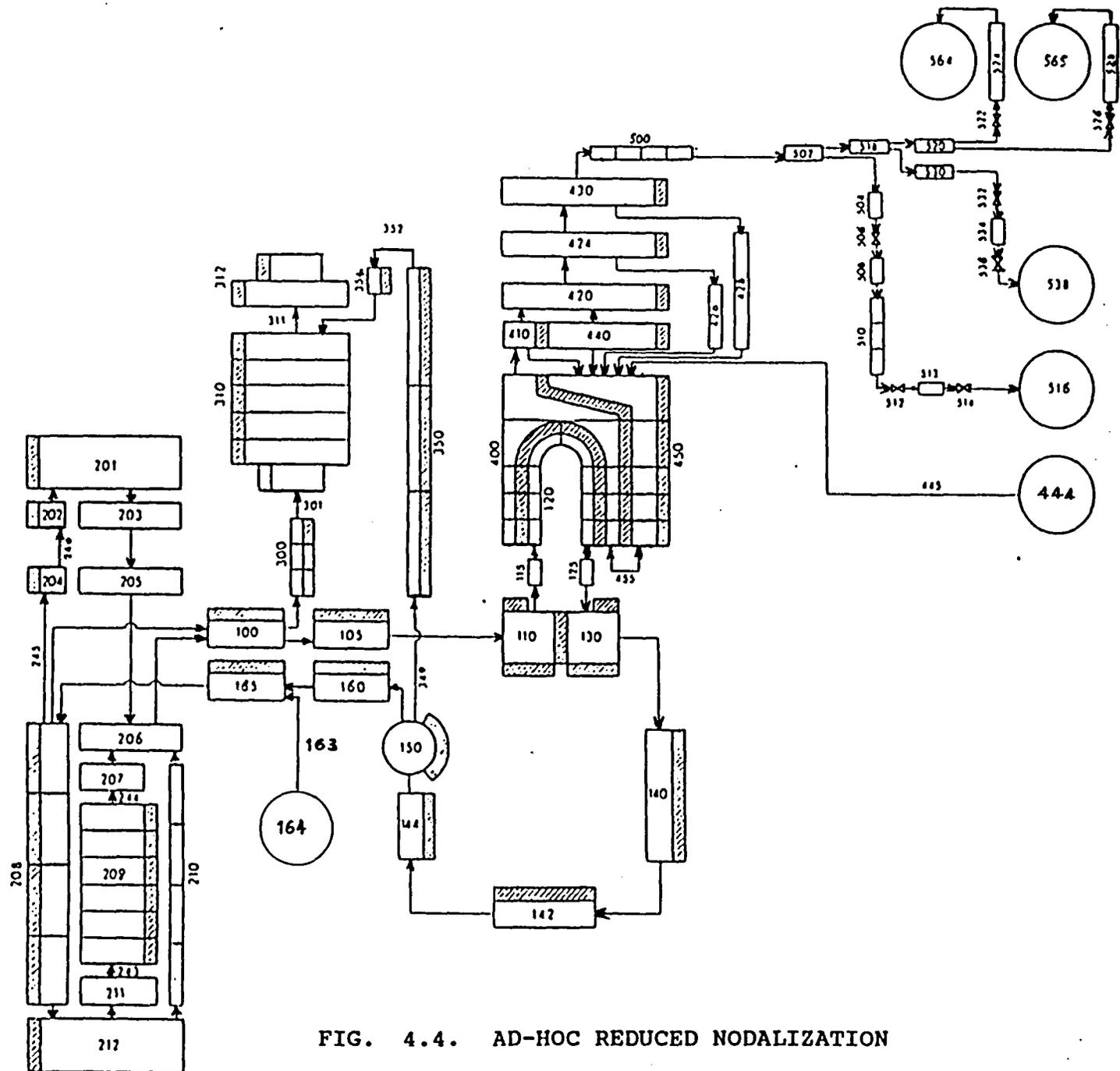
FIG. 4.4. AD-HOC REDUCED NODALIZATION
