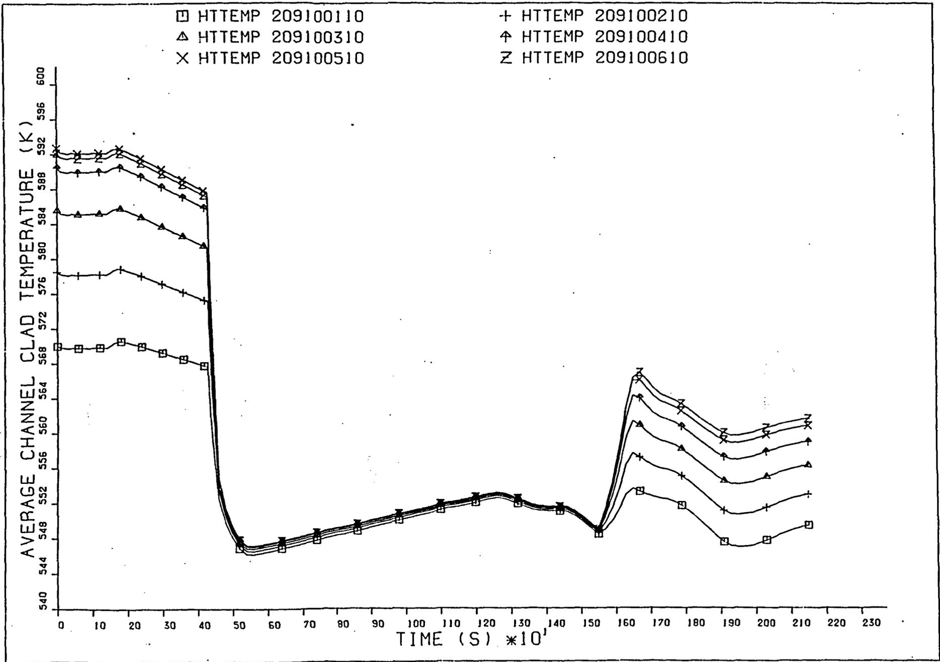
UNION-FENOSA ICAP INADVERTED PRZ SPRAY TOTAL. OPFNING (FIG 6.15)
