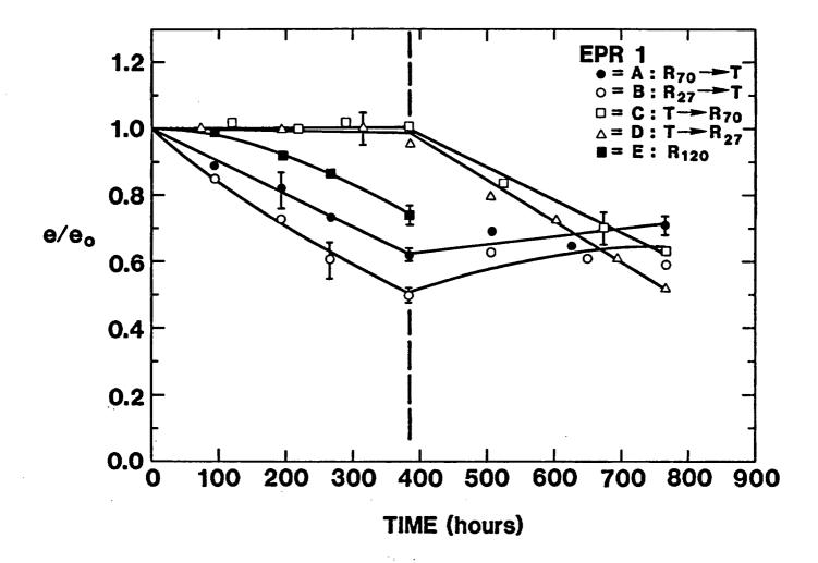
Figure 5.8. Ultimate Tensile Elongation of EPR 1 in Various Environments. Sample tensile elongation divided by initial (unaged) elongation is plotted versus aging time. Each portion of the sequential exposures lasted ~380 h.
