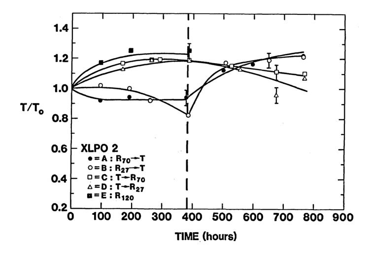
Figure 5.15. Ultimate Tensile Strength of XLPO 2 in Various Environments. Sample tensile strength divided by initial (unaged) strength is plotted versus aging time. Each portion of the sequential exposures lasted ~380 h.
