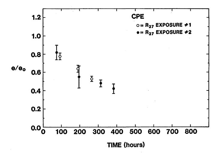
Figure 5.6. Repeatability of Ultimate Tensile Elongation Results for CPE During Two R<sub>27</sub> Exposures
