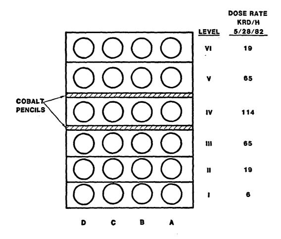
Figure 3.2. Arrangement of the Low Intensity Cobalt Array (LICA) facility for U.S./French aging program. French samples were aged using positions IV A-IV D. U.S. Samples were aged using positions III A-III D and V A-V D.
