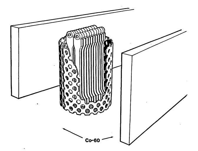
Figure 4.5. Orientation of 82 H5 and 82 H6 Samples During Irradiation
