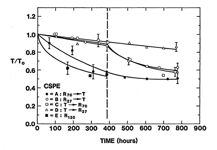
Figure 5.2. Ultimate Tensile Strength of CSPE in Various Environments. Sample tensile strength divided by initial (unaged) strength is plotted versus aging time. Each portion of the sequential exposures lasted ~380 h.
