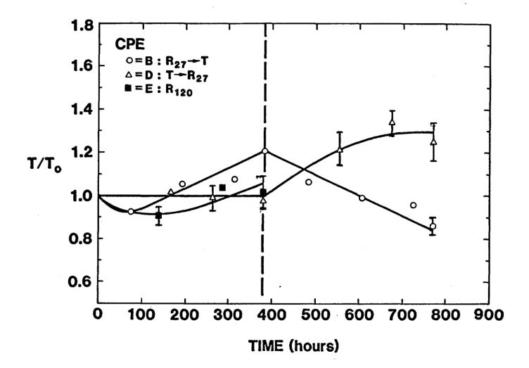
Figure 5.4. Ultimate Tensile Strength of CPE in Various Environments. Sample tensile strength divided by initial (unaged) strength is plotted versus aging time. Each portion of the sequential exposures lasted ~380 h.
