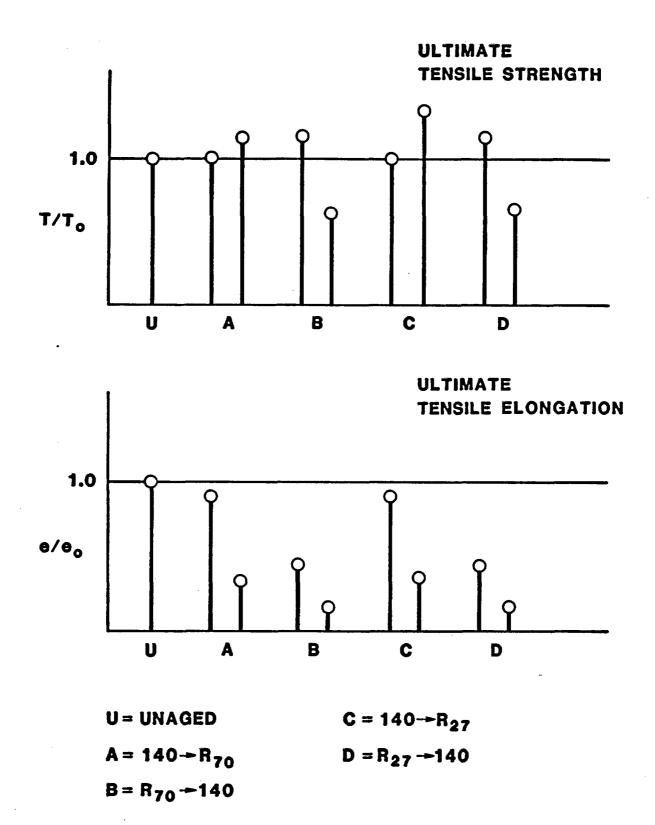
Figure 5.18. Ultimate Tensile Properties for Fire-proof EPDM (82 I9)
