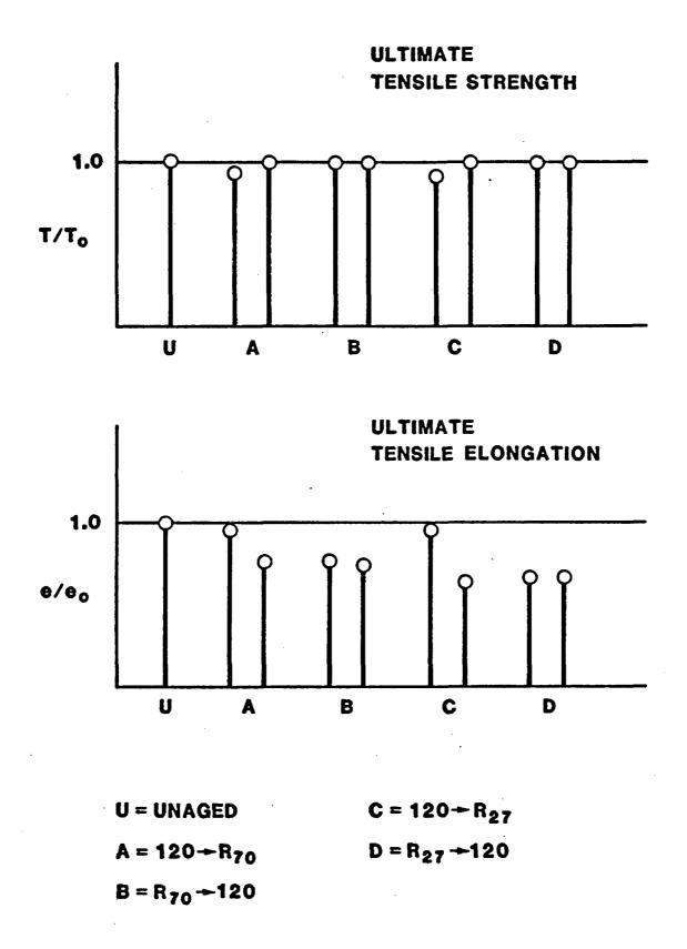
Figure 5.21. Ultimate Tensile Properties for VAMAC (82 H3)
