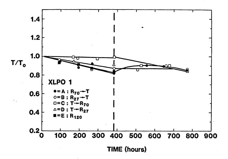
Figure 5.13. Ultimate Tensile Strength of XLPO 1 in Various Environments. Sample tensile strength divided by initial (unaged) strength is plotted versus aging time. Each portion of the sequential exposures lasted ~380 h.
