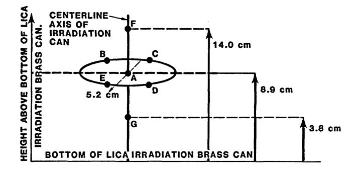
Figure 3.3. Locations of thermoluminescent  $CaF_2$  wafers inside LICA irradiation can during dose rate gradient mapping.  $CaF_2$  wafers were placed at Positions A, B, C, D, E, F, and G.
