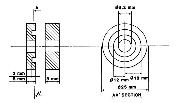
Figure 2.2. Compression Set Fixtures Used for 82 J3 and 82 J4 French O-ring Seal Samples
