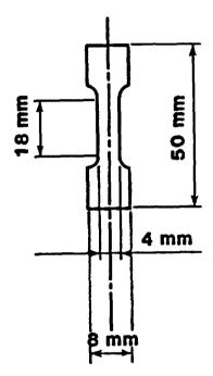
Figure 2.1. Dimensions for 82 GlO, 82 H3, and 82 H4 French Dumbbell Samples - H3 French Standard (Commission of Normalization N<sup>O</sup> NF.T 51-034-June 1968)
