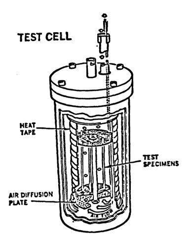
Figure 3.4. A LICA Irradiation Test Cell
