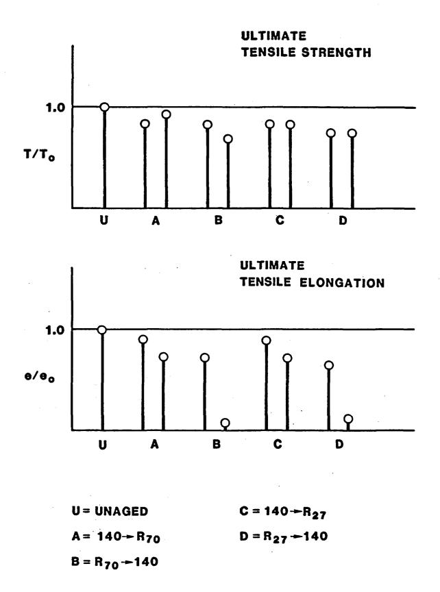
Figure 5.16. Ultimate Tensile Properties for PRC (82 Il)
