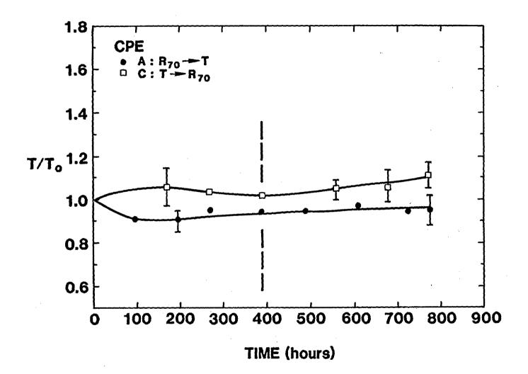
Figure 5.5. Ultimate Tensile Strength of CPE in Various Environments. Sample tensile strength divided by initial (unaged) strength is plotted versus aging time. Each portion of the sequential exposures lasted ~380 h.
