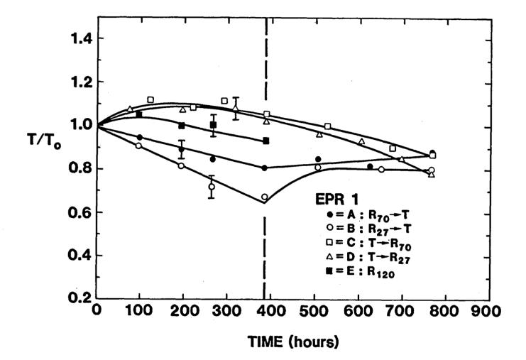
Figure 5.9. Ultimate Tensile Strength of EPR 1 in Various Environments. Sample tensile strength divided by initial (unaged) strength is plotted versus aging time. Each portion of the sequential exposures lasted ~380 h.
