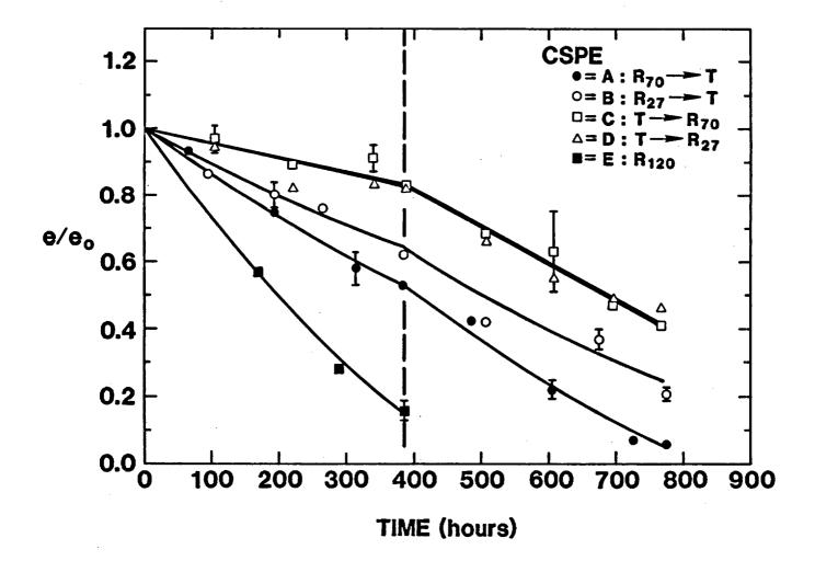
Figure 5.1. Ultimate Tensile Elongation of CSPE in Various Environments. Sample tensile elongation divided by initial (unaged) elongation is plotted versus aging time. Each portion of the sequential exposures lasted ~380 h.
