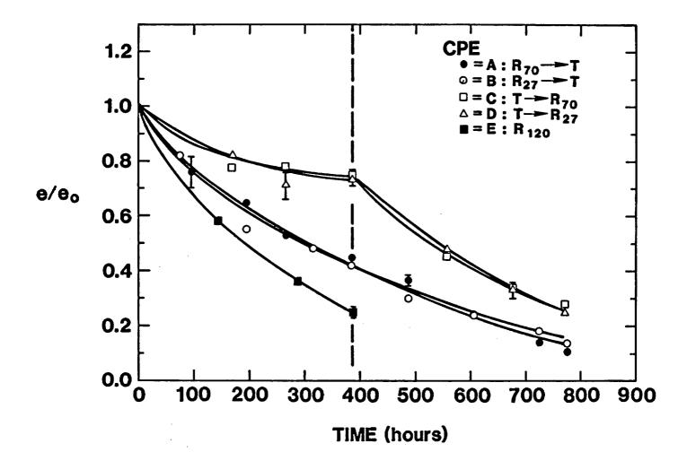
Figure 5.3. Ultimate Tensile Elongation of CPE in Various Environments. Sample tensile elongation divided by initial (unaged) elongation is plotted versus aging time. Each portion of the sequential exposures lasted ~380 h.
