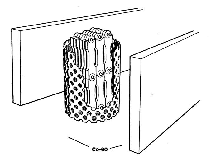
Figure 4.8. Orientation of 82 H3, 82 H4, and 82 G10 Samples During Irradiation
