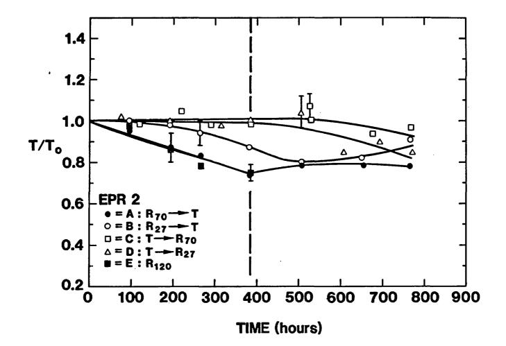
Figure 5.11. Ultimate Tensile Strength of EPR 2 in Various Environments. Sample tensile strength divided by initial (unaged) strength is plotted versus aging time. Each portion of the sequential exposures lasted ~380 h.
