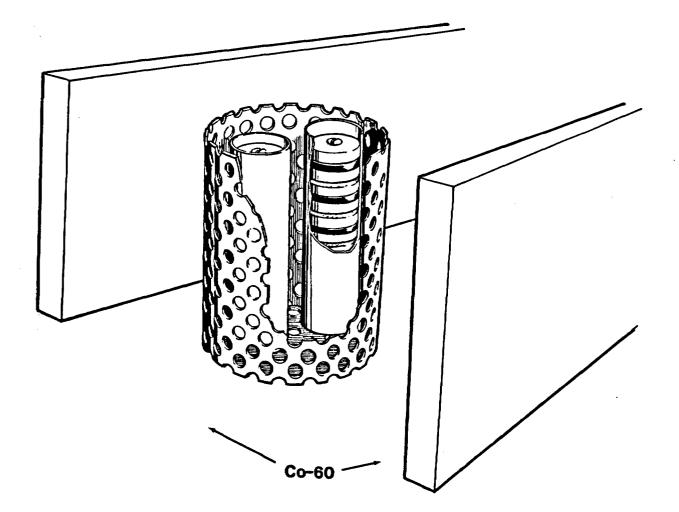
Figure 4.10. Irradiation Aging Configuration Used for 82 J4 Samples
