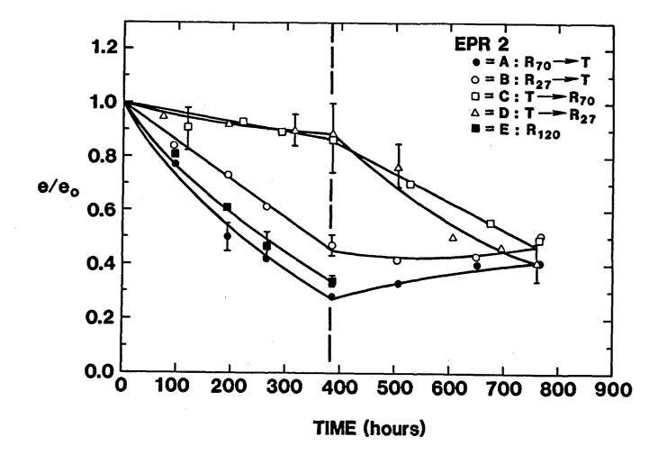
Figure 5.10. Ultimate Tensile Elongation of EPR 2 in Various Environments. Sample tensile elongation divided by initial (unaged) elongation is plotted versus aging time. Each portion of the sequential exposures lasted ~380 h.
