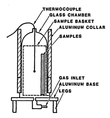
Figure 3.6. Oven Aging Cell
