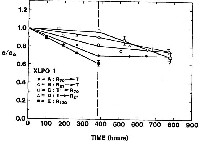
Figure 5.12. Ultimate Tensile Elongation of XLPO 1 in Various Environments. Sample tensile elongation divided by initial (unaged) elongation is plotted versus aging time. Each portion of the sequential exposures lasted ~380 h.
