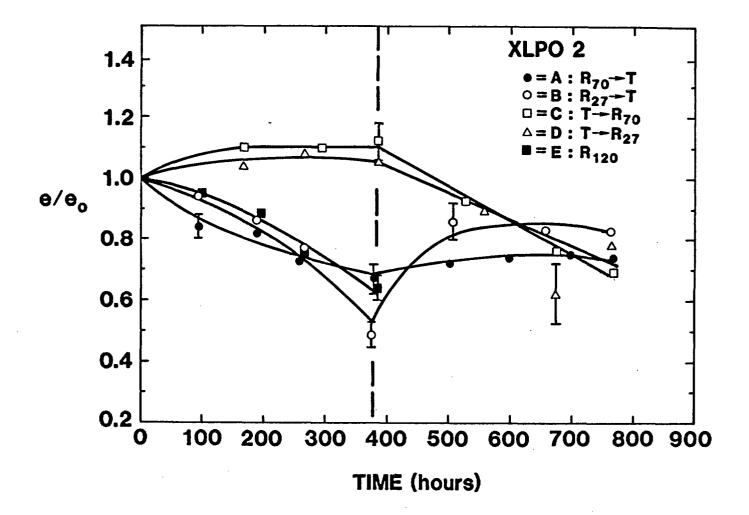
Figure 5.14. Ultimate Tensile Elongation of XLPO 2 in Various Environments. Sample tensile elongation divided by initial (unaged) elongation is plotted versus aging time. Each portion of the sequential exposures lasted ~380 h.
