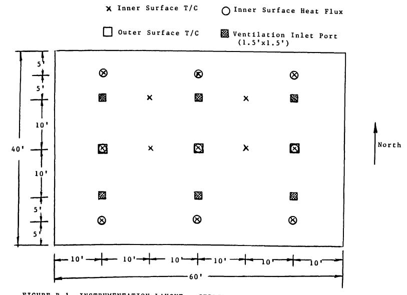
FIGURE B-1 INSTRUMENTATION LAYOUT - CEILING (View looking into enclosure)
