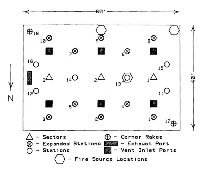
Figure 2: Placement of instrument trees within the test enclosure.
