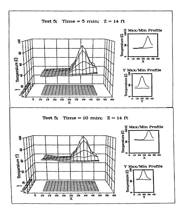
Figure 9: Three-Dimensional Plot of Temperature Versus Plan View Location for the 14-Foot Elevation at 5 and 10 Minutes After Ignition in Test 5.
