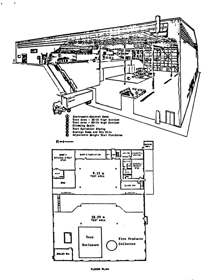
FIGURE A-1 FM TEST CENTER (TOP) AND TEST ENCLOSURE LOCATION (BOTTOM)
