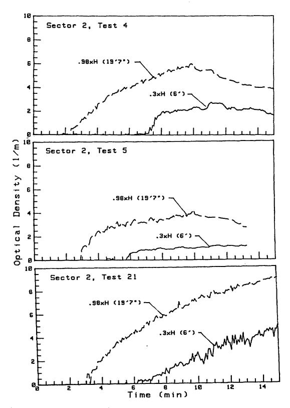
Figure 12: Smoke Optical Density to Blue Light at Each of Two Elevations on Sector 2 Instrument Tree During Tests 4, 5, and 21.
