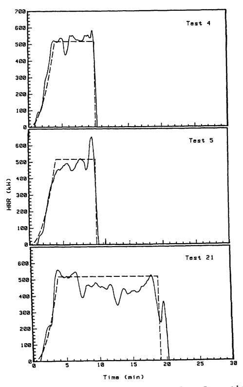
Figure 6: Heat Release Rates Calculated Based on Generation Rate of Carbon Dioxide for Tests 4, 5, and 21.
