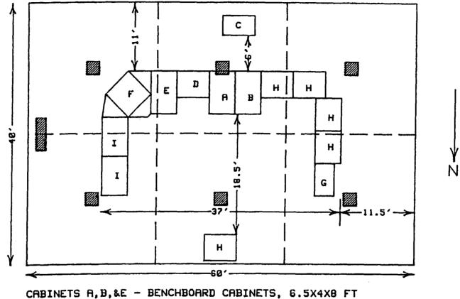
CABINETS H, B, & E - BENCHBOARD CHBINETS, 5.5X4X8 FT CABINET F - MITERED BENCHBOARD CABINET, 6.5X6.5X8 FT CABINETS C&G - VERTICAL CABINETS, 3X5X7.5 FT CABINETS D&H - CABINET MOCKUPS, 4X5X8 FT CABINETS I - CABINET MOCKUPS, 4X6X8 FT
