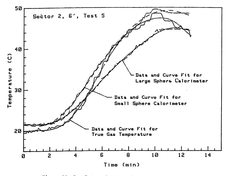
Figure 18: Raw Data and Curve Fit for Sector 2, 6 Foot Location Sphere Calorimeter Processing During Test 5.
