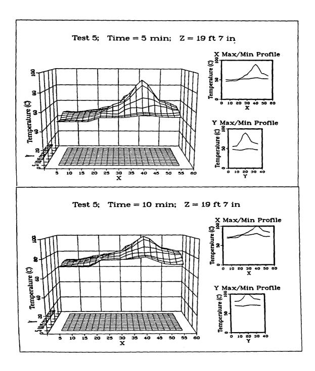
Figure 11: Three-Dimensional Plot of Temperature Versus Plan View Location for the 19-Foot. 7-Inch Elevation at 5 and 10 Minutes After Ignition in Test 5.
