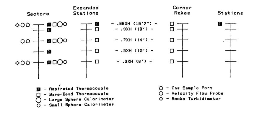
Figure 3: Definition of instrumentation on each of the instrument tree types shown in Figure 2.
