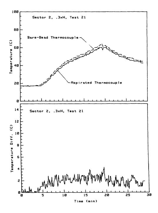
Figure 17: Data From Bare-Bead and Aspirated Thermocouples at Section 2, 6-Foot Location During Test 21.
