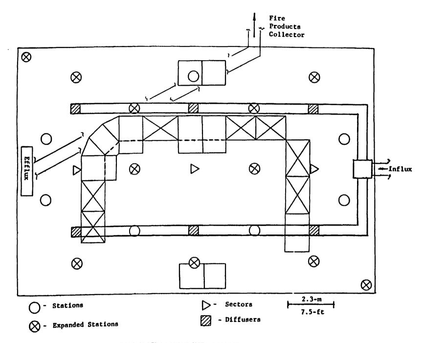
FIGURE A-3 VENTILATION SYSTEM LAYOUT WITH RESPECT TO INSTRUMENTATION AND CABINETS
