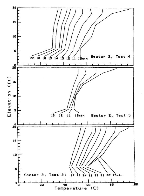
Figure 14: Vertical Temperature Profiles at Sector 2 Location Following Fire Extinguishment in Tests 4, 5, and 21.
