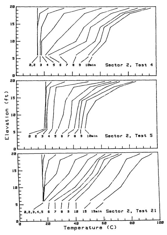
Figure 13: Vertical Temperature Profile at Sector 2 Location During Fire Growth and Fire Steady-State Periods of Tests 4, 5, and 21.
