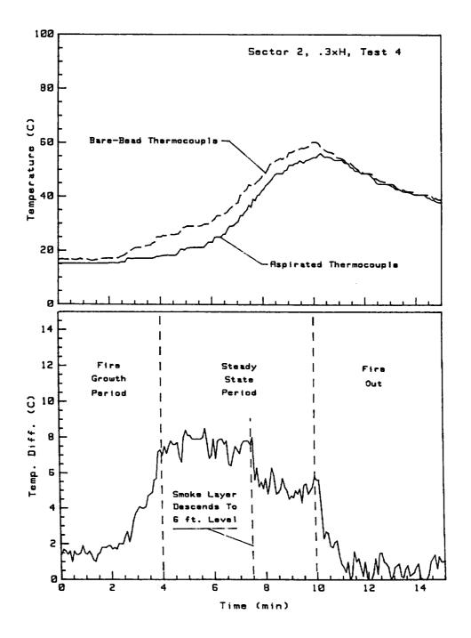
Figure 15: Data From Bare-Bead and Aspirated Thermocouples at Section 2, 6-Foot Location During Test 4.
