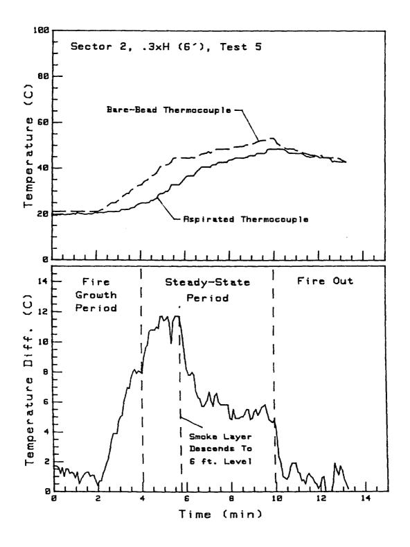
Figure 16: Data From Bare-Bead and Aspirated Thermocouples at Section 2, 6-Foot Location During Test 5.
