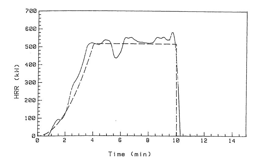
Figure C-2: Actual burner profile and calculated heat release rate for Test 4.
