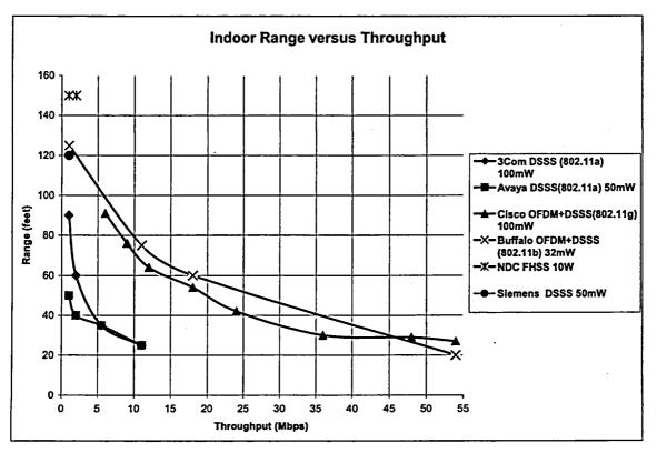
Figure 4.3. Graph of throughput vs range for different output powers.
