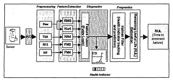
Figure 5.3. Processing flow for the CCP smart sensor. (reproduced with permission).
