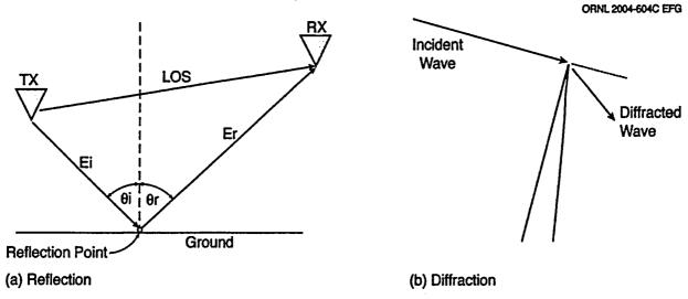
Figure 4.1. Reflection and diffraction.
