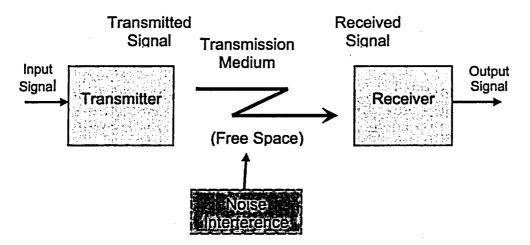
Figure 2.1. Elements of a wireless system.
