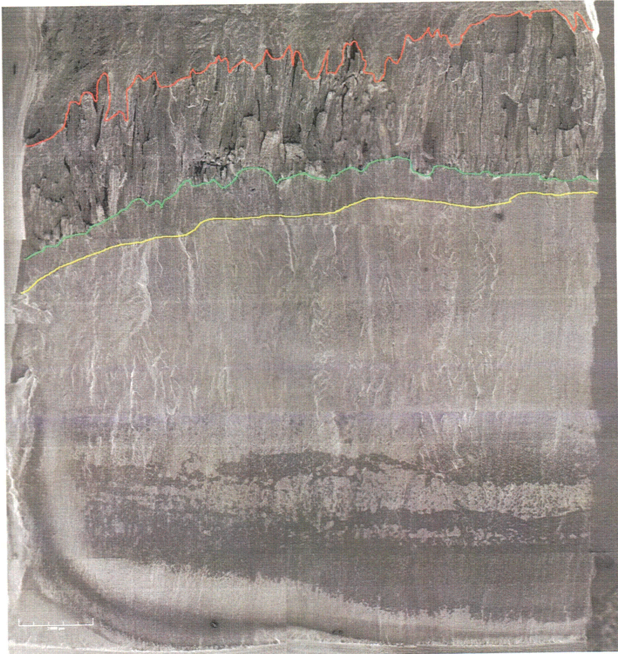
Figure 35. Fracture surface of specimen CT31-W02 TS. Crack extension from bottom to top of the figure.
