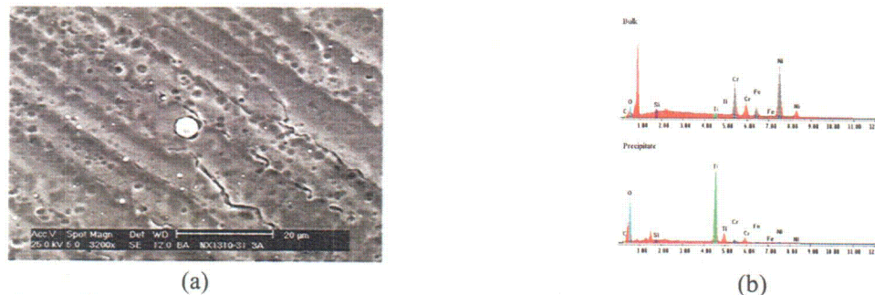
Figure 14. (a) Micrograph showing one of the matrix precipitates observed on the surface of sample 3A and (b) EDX spectra resulting from the bulk and the precipitate shown in (a).
