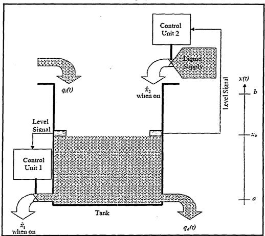
Figure 1.6 A Level Controller with 2 On/Off Controllers
