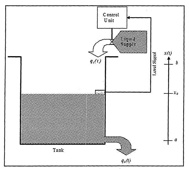
Figure 1.7 A Level Controller with 1 Proportional Controller
