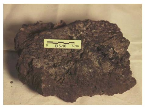
Figure 1-4. Hand sample of Site B slag. This sample is more crystalline the one shown in Figure 1-3 indicating that it was from the interior of a melt block. (Photograph courtesy of CNWRA).
