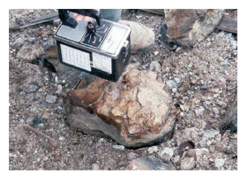
Figure 1-6. Close up of slag found at the ground surface at Site C. The interior is medium gray in color. The outer rusty brown colored surface is indicative of the rapid weathering of these blocks when exposed to the atmosphere.
