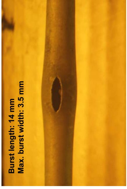
ICL#2: LOCA sequence with 5-minute oxidation at 1204°C and slow-furnace cooling
