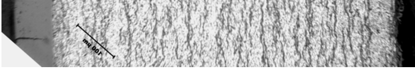
HBR C11 Annealed Uniform Circumferential Hydrides
