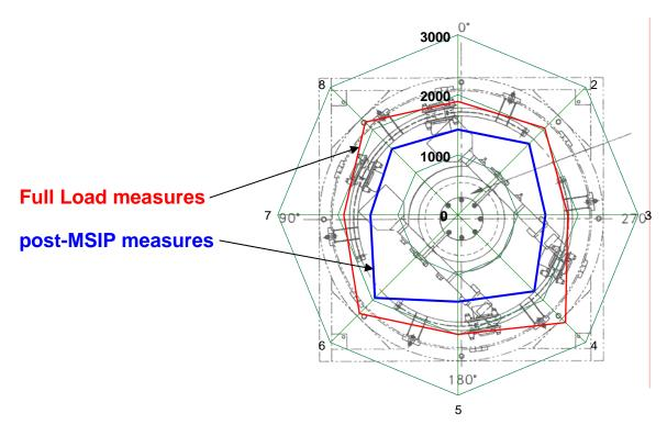
Figure 7 - Polar Plot of Hoop Strains (Micro-Inches per Inch)
