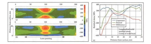
Figure 5. Residual Stress in a 33-mm Thick Alloy 22 Welded Plate: (a) Map of Residual Stress in Unpeened Weld; (b) Map of Residual Stress in Laser Peened Weld; (c) Line Plot of Residual Stress Versus Depth at the Center of the Weld Bead,
