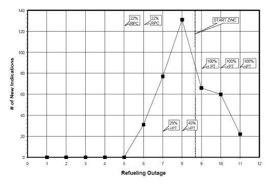
**<u>Figure 7</u>** Example of field data from Diablo Canyon Unit 1: new indications of PWSCC at tube-support-plate (TSP) locations
