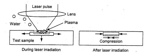
Figure 4. Typical Laser Peening Process.
