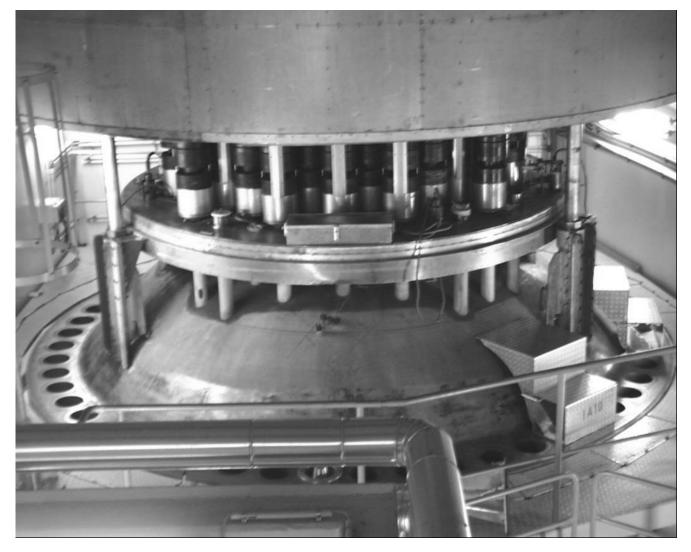
Figure 10 RPV head on its storage location during outage
