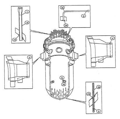
Fig.1 Alloy 600 components of the RV pressure boundary
