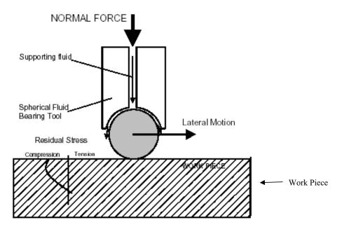
Figure 7. Low Plasticity Burnishing Schematic.
