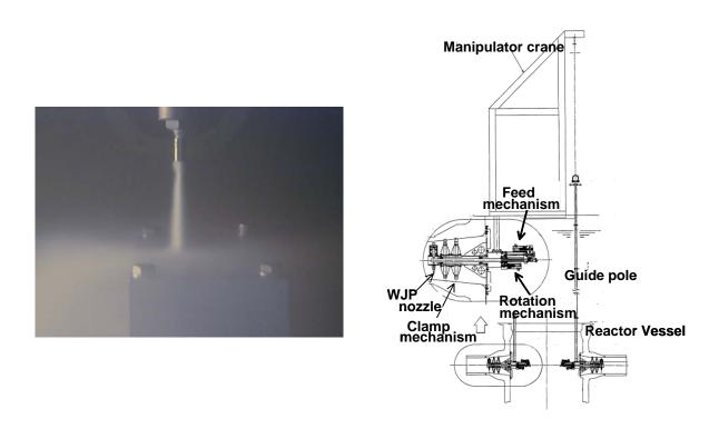
Fig.5 Concept of WJP for outlet/inlet nozzle safe ends
