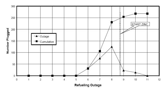
Figure 6Example of field data from Diablo Canyon Unit 1:<br/>plugging for PWSCC at tube-support-plate (TSP) locations
