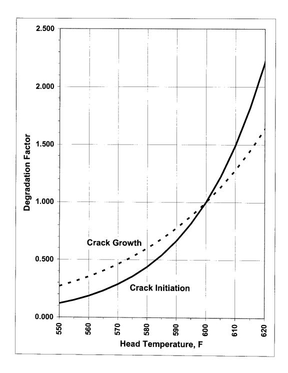
Figure 4: Degradation Factor as a Function of Temperature
