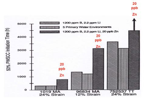
Figure 4Example for the effect of zinc on time to initiate PWSCC in<br/>laboratory tests (after Esposito et al. [1])
