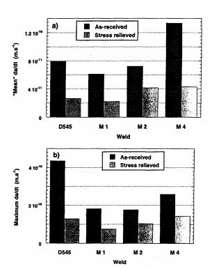
Figure 3 Effects of heat treatment on SCC susceptibility of Alloy 182 [2], results of CGR tests carried out in primary water at 330 °C and an initial K<sub>I</sub> of 20 MPaKm
