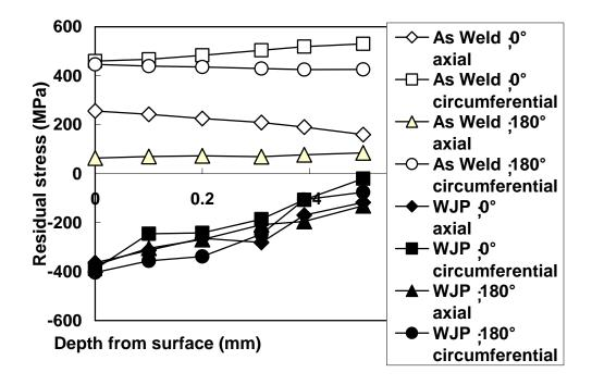
Fig.3 Results of residual stress measurement before and after WJP
