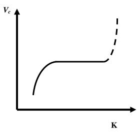
Figure 4, Sketch of the general appearance of an environmentally assisted cracking process with respect to some crack driving force, in this case the stress intensity level K.
