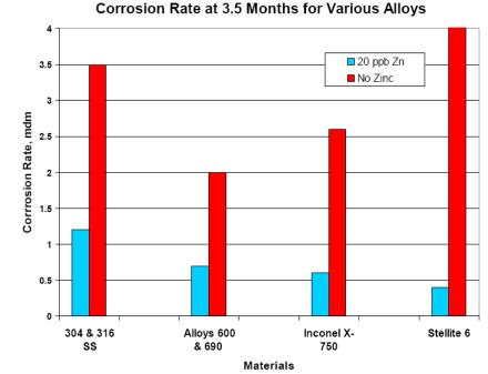
**Figure 3** Effect of zinc on corrosion rates of various alloys in laboratory tests (after Esposito et al. [1])
