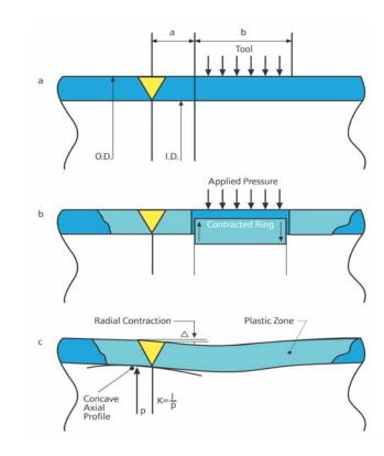
**Figure 1 – Schematic Illustration of MSIP Process**
