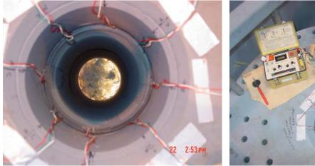
Figure 4(a) Illustration of the Instrumented Strain Gauges Installed on the ID Surface Near the Weld Location of the Mockup Pressurizer Nozzle
