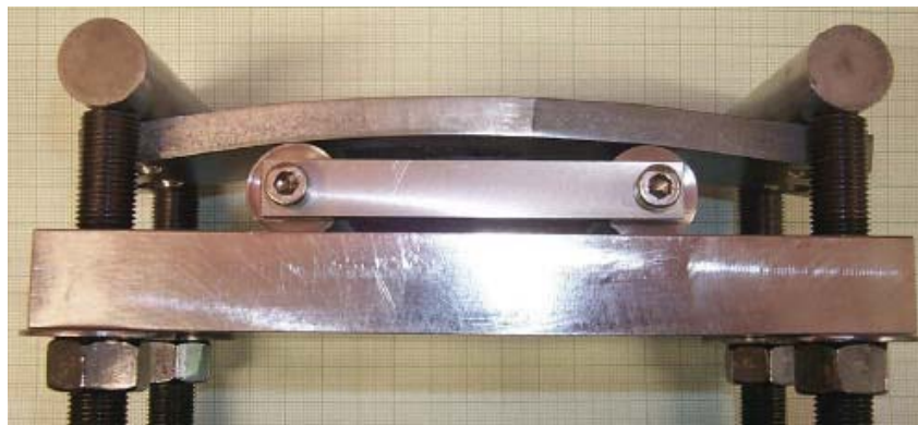
Figure 1 - Photographs of Alloy 52M (Upper 1 thru 4), Alloy 600 (600-1 thru-4), and Alloy 182- 4 (lower photo) bent beam test specimens. [Specimens with suffixes -1 and -2 were strained 0.35%; those with suffixes -3 and -4 wee strained 1.0%]
