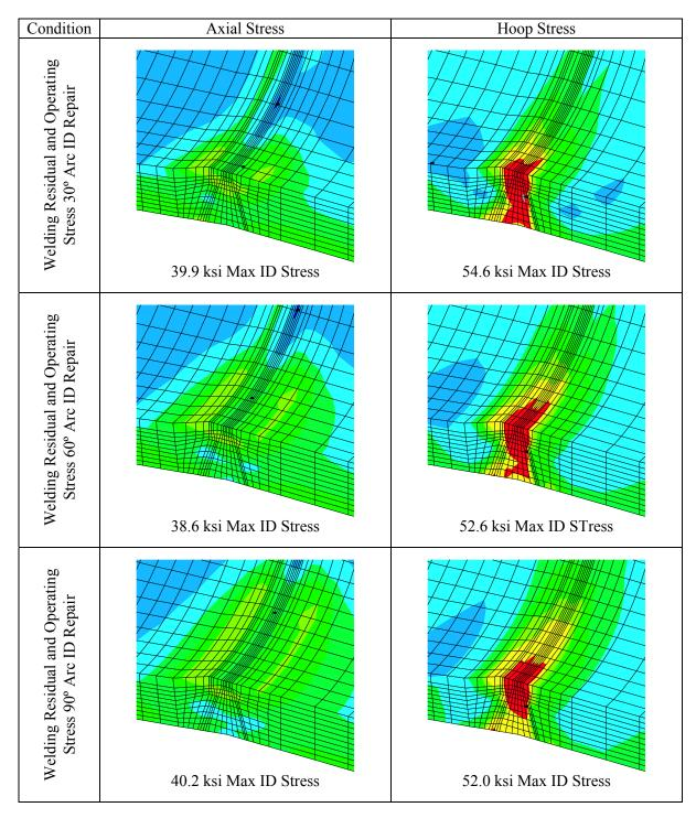
Figure 9 Welding Residual and Operating Stresses With Partial-Arc ID Weld Repairs
