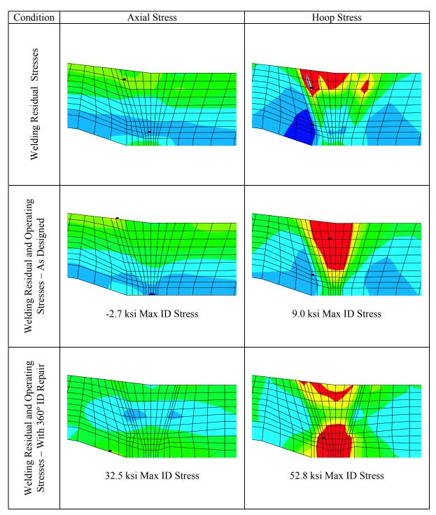
Figure 8 Welding Residual and Operating Stresses With and Without 360° ID Weld Repair
