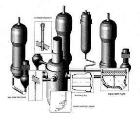
Fig 4 : Inconel components in primary system
