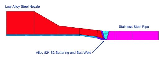
Figure 6 Pressurizer Surge Nozzle – Mesh in Area of Weld and Overlay
