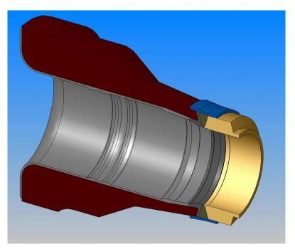
Figure 5 Pressurizer Surge Nozzle – Overall Finite Element Model
