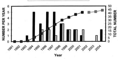
Fig. 7 : Vessel head replacement since 1993
