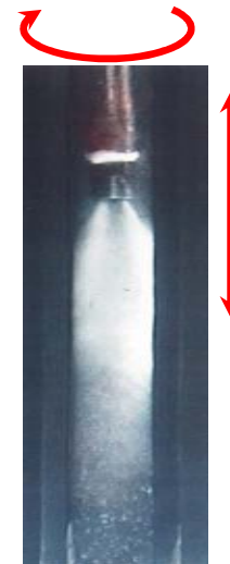
State of WJP in small diameter pipe
