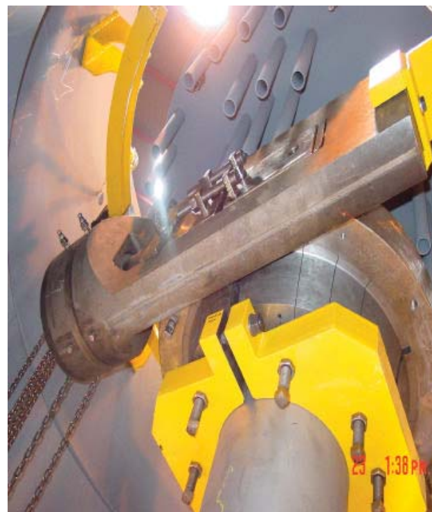
Pressurizer Surge Nozzle Mock-up for Tihange 2
