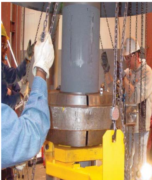
Pressurizer Surge Nozzle Mock-up for Tihange 2
