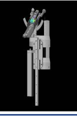
•"Grooveman" is used to perform eddy current inspections of the J-weld and penetration tube OD surface
