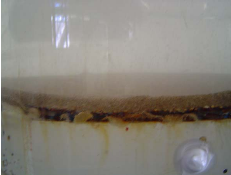
Fig. 51. Test 16 debris bed of common sand.
