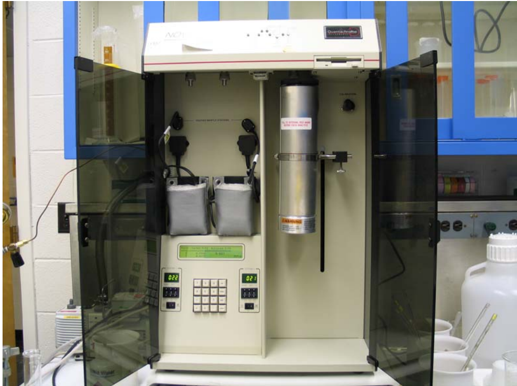
Fig. 29. Nitrogen adsorption BET instrumentation.
