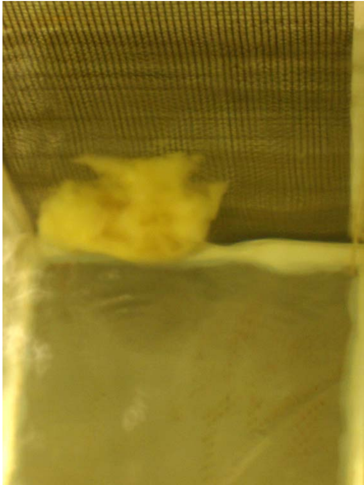
Figure 7-1 NUKON™ That Is Tested Directly after Being Processed from a Leaf Shredder Forms Clusters at the Test Screen
