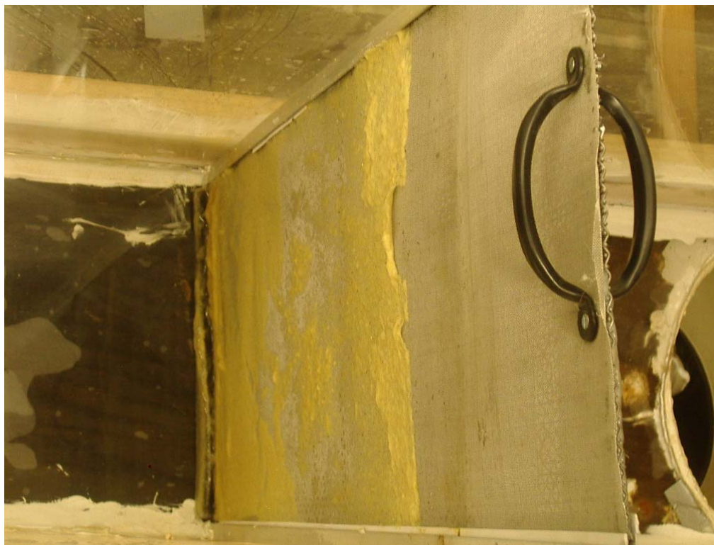
Figure 5-4 Finer-Sized NUKON™ Collected on the Fine Screen Located Downstream
