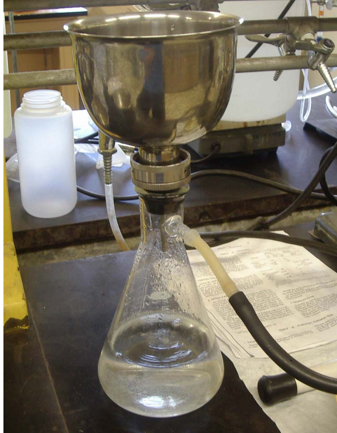
Figure 4-1 Filtration of NUKON™ To Remove Water
