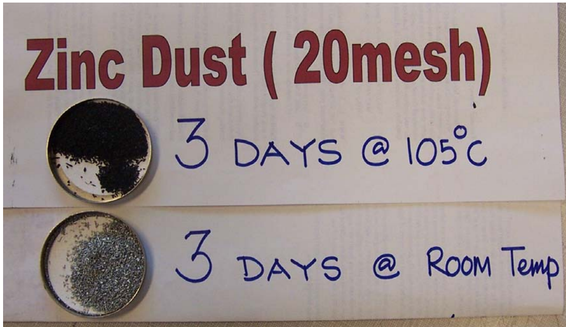
Figure 5-11. Zinc granules after 3 days in oven at 105° C and at room temperature at a pH of about 7.
