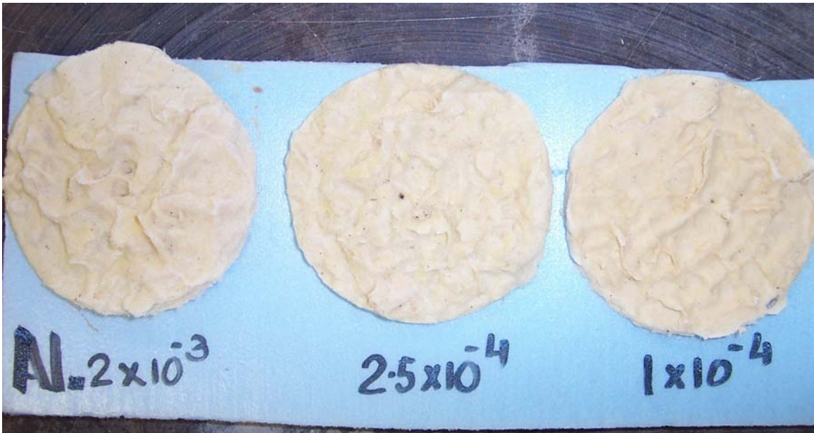
Figure 4-11. Bed with precipitates of aluminum nitrates at different concentrations.
