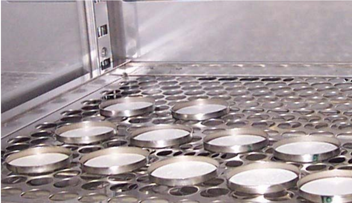
Figure 5-7. 45- \mu\text{m} glass-filter paper being oven dried before filtration.
