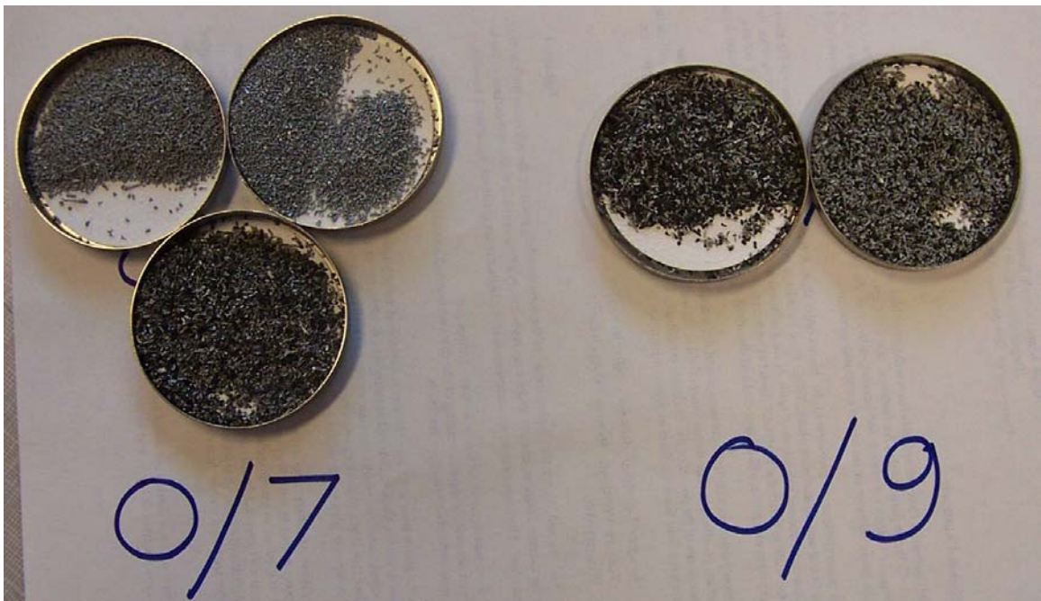
Figure 5-10. Zinc granules after exposure in oven (O) for 7 days at pHs of 7 and 9.
