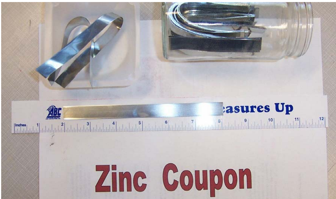
Figure 5-2. Unreacted zinc coupon (15.3 cm × 1.3 cm × 0.67 mm).
