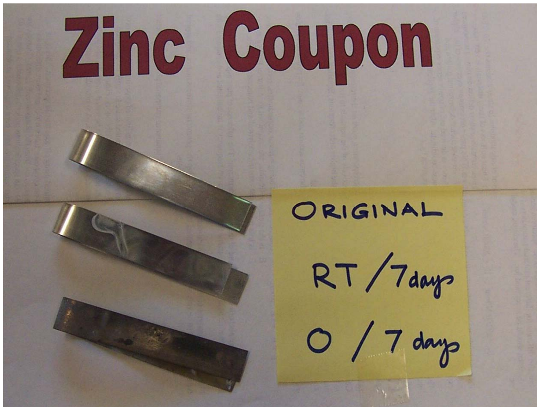
Figure 5-12. Zinc coupons before and after exposure at room temperature and in oven.
