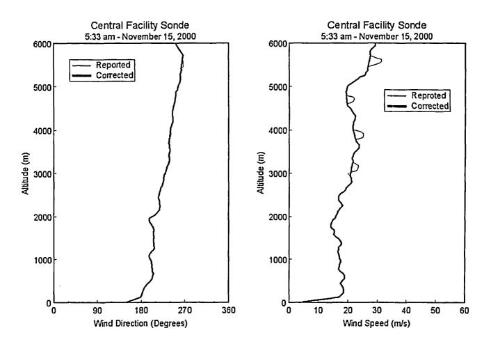
**Figure 7.** Central Facility Sonde Launched at 5:33 am CST on November 15, 2000. Quite a few of the sondes exhibited speed anomalies in an otherwise fairly smooth profile. They were often associated with a missing layer in the data. They were corrected by interpolating between the bottom and top of the anomaly. Note that direction was hardly affected.
