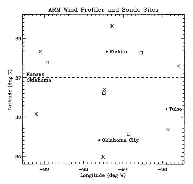
**Figure 2.** Location of ARM Upper Air Observations. + indicates sonde and AERI sites, × indicates NOAA Profiler sites, and  $\Box$  915 MHz RWP/RASS sites. Note that some sites have multiple measurements, and the Central Facility has all three types.
