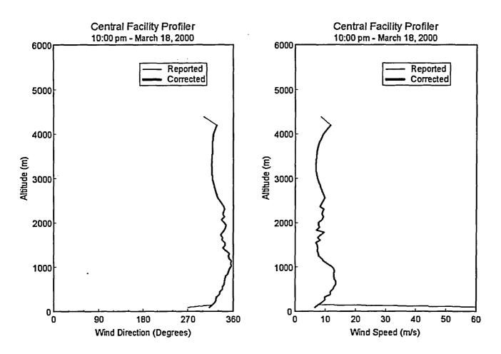
**Figure 6**. 915 MHz RWP Wind Profile for the Central Facility at 10:00 pm CST on March 18, 2000. This is an example case where the reported lowest level wind (77.5 m/s) is wrong. The corrected profile is determined by extrapolating downward from the 2 levels above. Where the two profiles overlap only the heavy line shows.
