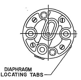
Figure 1. Diaphragm Locating Tabs
