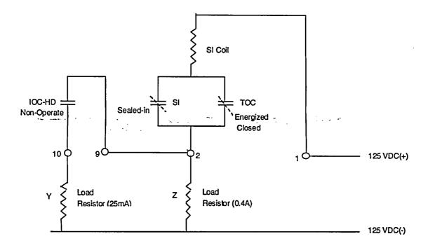
Figure 1. Alternate Output Monitoring Circuit
