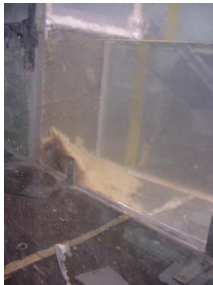
(iii) Pile of debris formed in front of the screen when flow through the flume was terminated.
