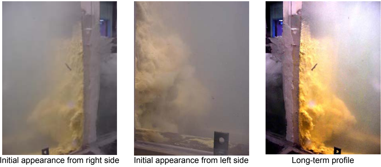
Figure B.1: The debris did not cover the entire width of the screen and left ~2 in. of space relatively open on one side, in addition to the 3 in. of opening at the top.
