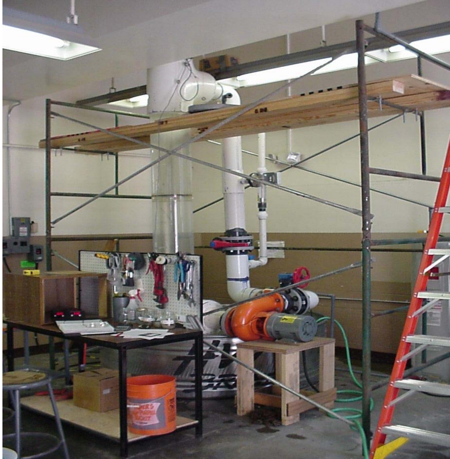
Figure A.8. UNM closed-loop head-loss test facility.
