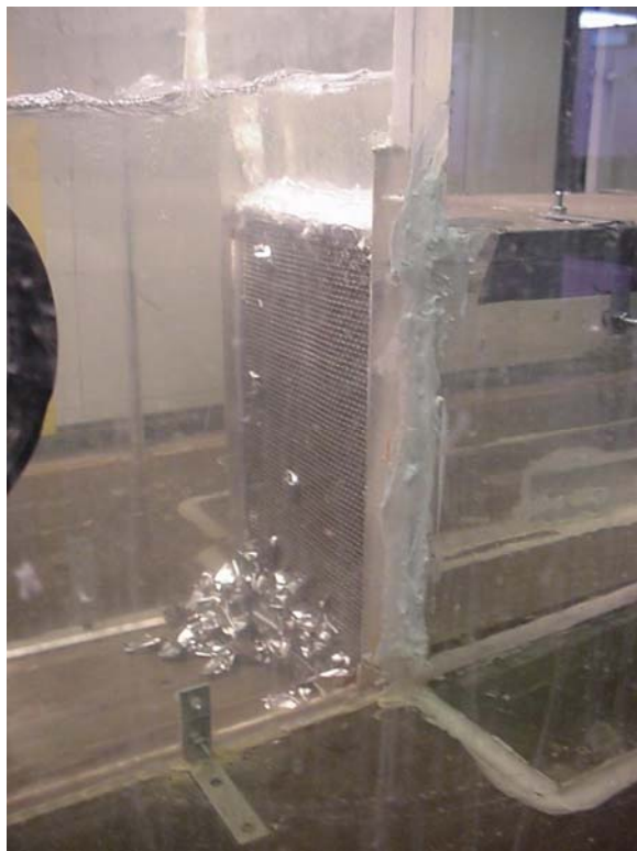
Figure B.4. RMI foil configuration after the initial 101.5 g was added (left), then several min later when a second 101.5 g was added (right).
