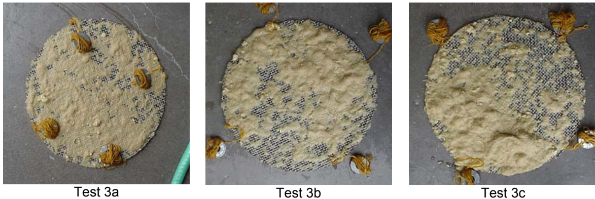
Figure 3.13. Post-test debris distribution on horizontal screens in thin-bed mixed debris Tests 3a-c.
