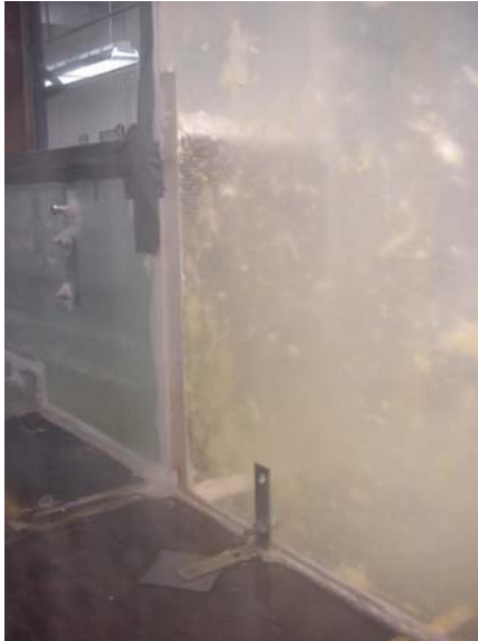
(i) Debris transport and accumulation on screen.
