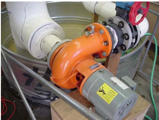
Figure A.11. 5-hp motor at the base of the vertical test section of the hydraulic loop.
