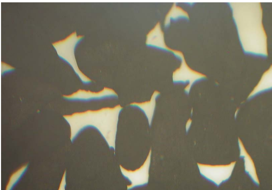
Fig. 5-20. Zinc granules after exposure (oven at 105° C for 3 days) under optical microscope (magnification 49).
