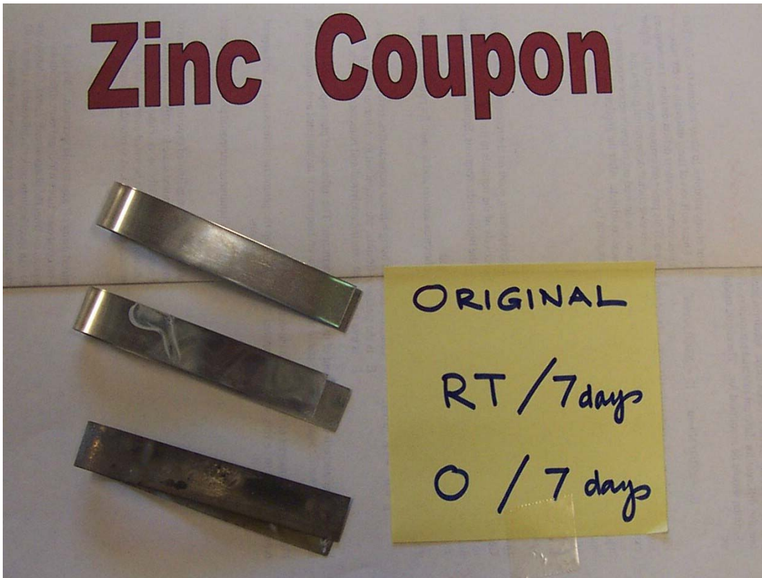
Fig. 5-12. Zinc coupons before and after exposure at room temperature and in oven.
