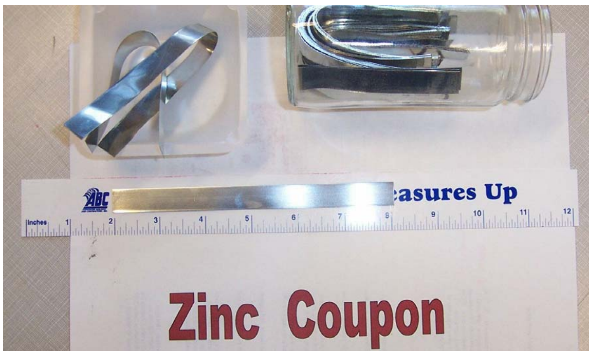
Fig. 5-2. Unreacted zinc coupon (15.3 cm × 1.3 cm × 0.67 mm).
