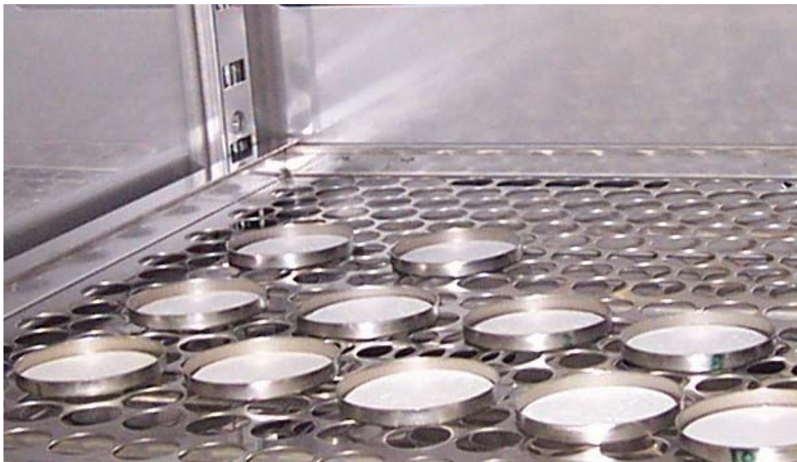
Fig. 5-7. 45- \mu m glass-filter paper being oven dried before filtration.
