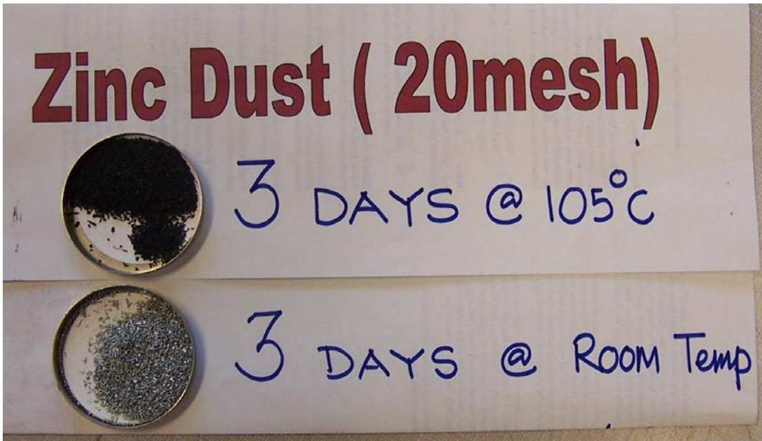
Fig. 5-11. Zinc granules after 3 days in oven at 105° C and at room temperature at a pH of about 7.
