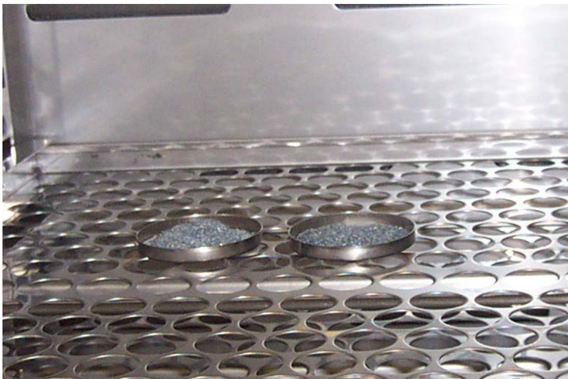
Fig. 5-8. After-filtration samples being dried.
