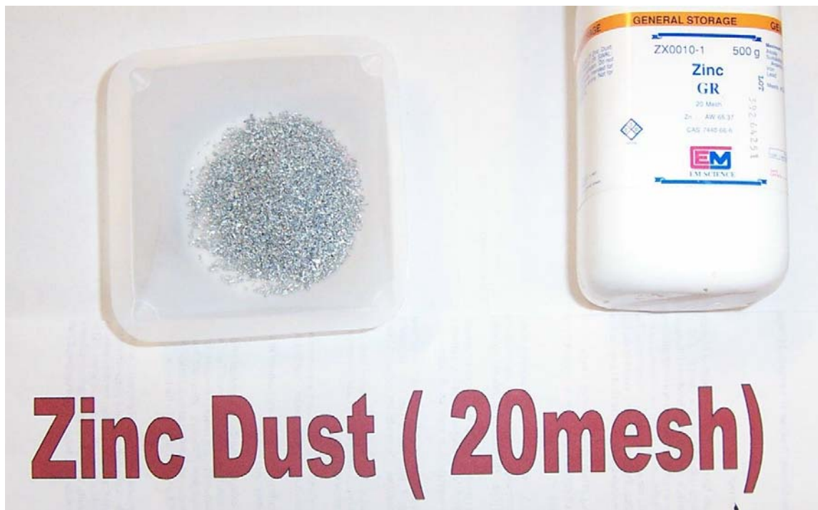
Fig. 5-1. Unreacted zinc granules (20 mesh).
