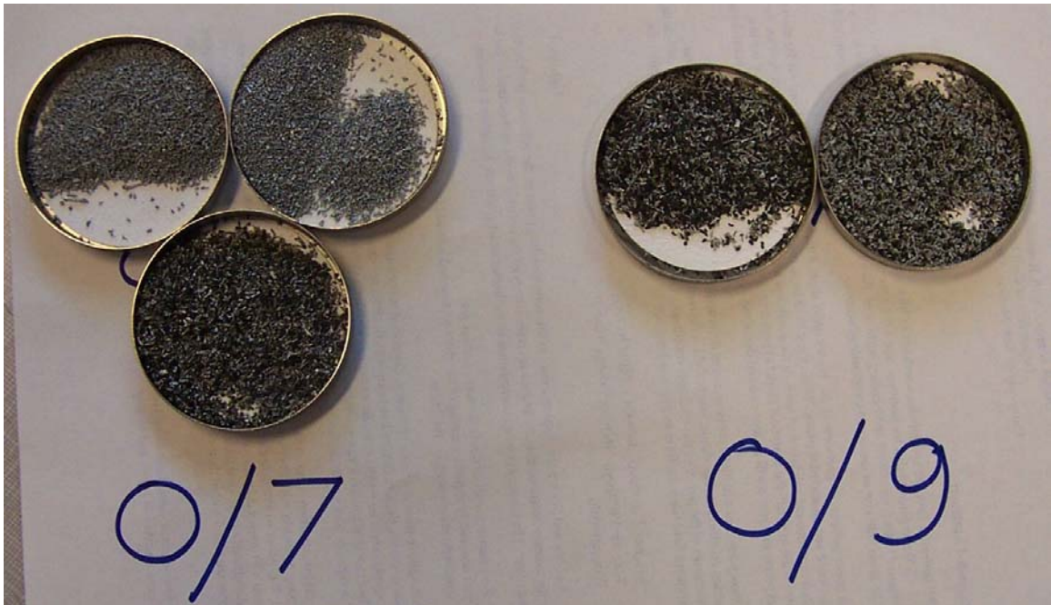
Fig. 5-10. Zinc granules after exposure in oven (O) for 7 days at pHs of 7 and 9.
