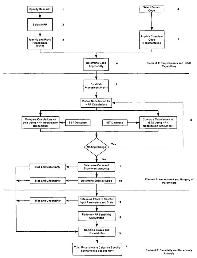
Figure II.5 Illustration of the CSAU Methodology
