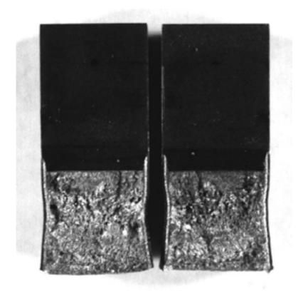
Figure A-2.2. Fracture surface of specimen Y4-02 tested at 288°C
